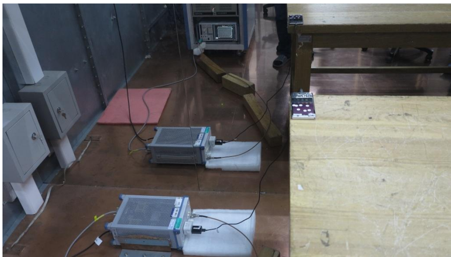
Picture C-4: Conducted Emissions Measurements
