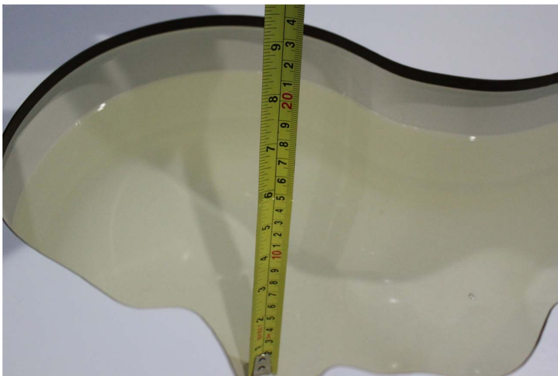
Picture 7-15 Liquid depth in the Head Phantom (5GHz)
