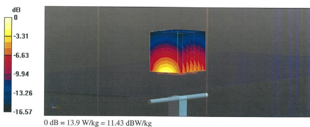
Impedance Measurement Plot for Body TSL
