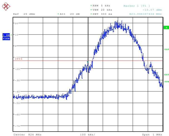
**HIGH BAND EDGE BLOCK-C (GSM850) –Channel 251**
