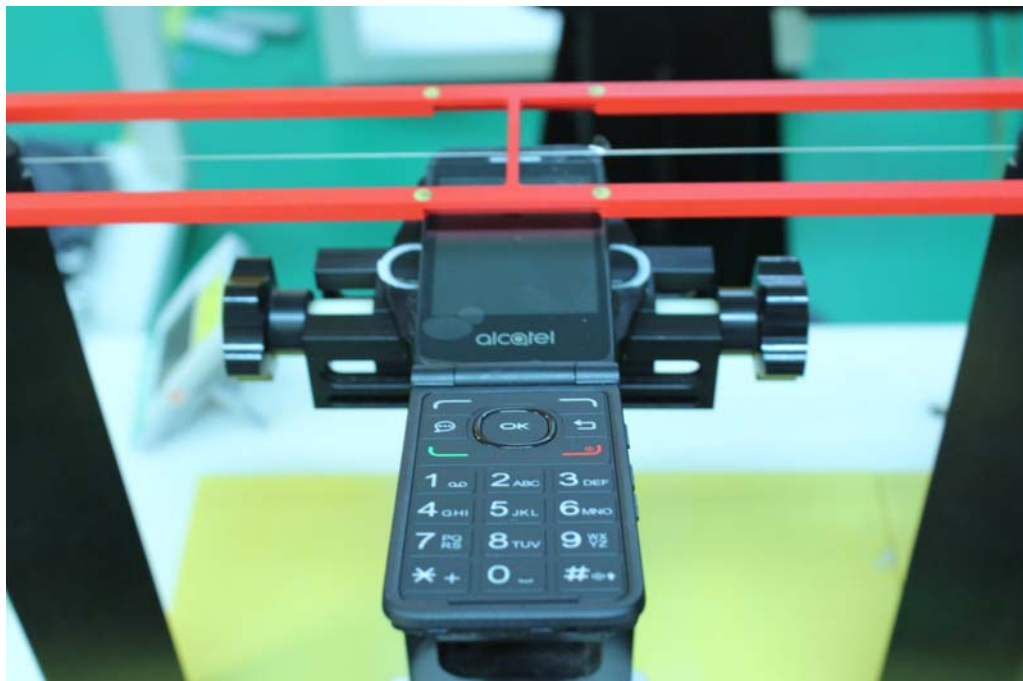
Picture 2: EUT Positioning for RF/T-coil
