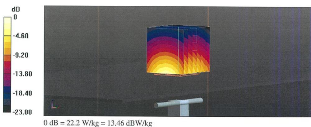
Impedance Measurement Plot for Head TSL
