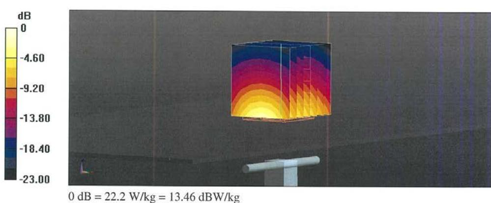
Impedance Measurement Plot for Head TSL
