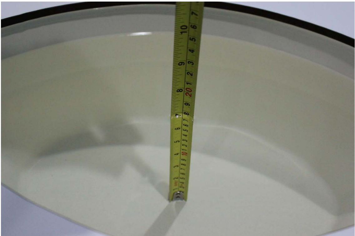
Picture 7-12 Liquid depth in the Flat Phantom (5GHz)
