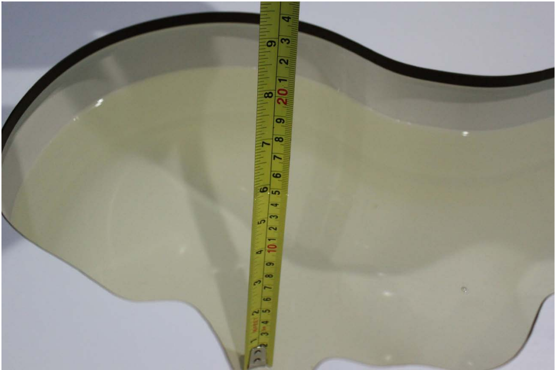
Picture 7-11 Liquid depth in the Head Phantom (5GHz)
