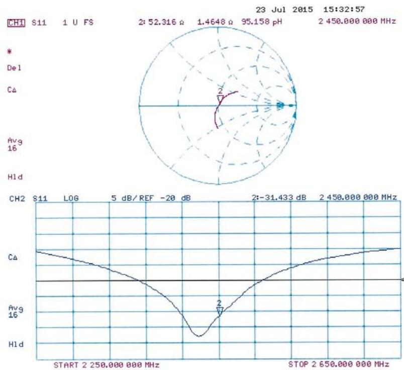
Impedance Measurement Plot for Body TSL
