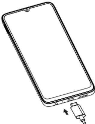
1. Insert the USB-C cable into the charge port as shown.
