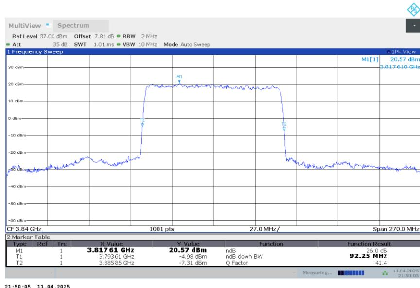
**n77H,90MHz Bandwidth,DFT-s-QPSK (-26dBc BW)**
