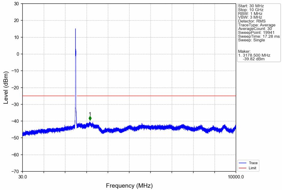
CA\_7C\_SISO\_NTNV\_CC1:10 CC2:20MHz\_CC1:QPSK CC2:QPSK\_CC1:2505 CC2:2519.4MHz\_CC1: 50@0 CC2: 100@0
