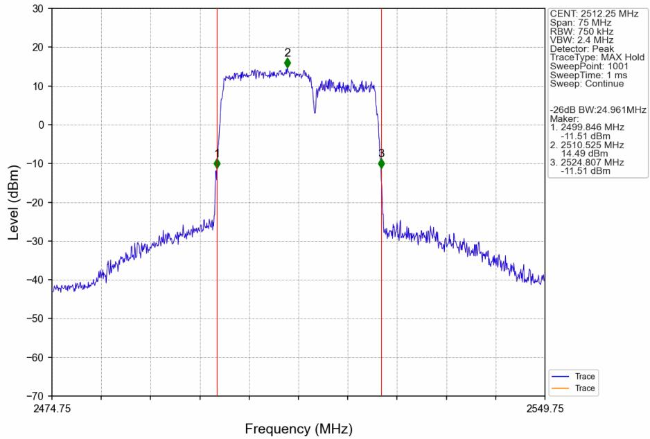
CA\_7C\_SISO\_NTNV\_CC1:15 CC2:10MHz\_CC1:256QAM CC2:256QAM\_CC1:2553 CC2:2565MHz\_CC1: 75@0 CC2: 50@0
