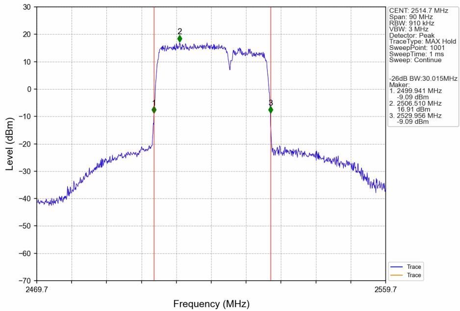
CA\_7C\_SISO\_NTNV\_CC1:20 CC2:10MHz\_CC1:QPSK CC2:QPSK\_CC1:2550.6 CC2:2565MHz\_CC1: 100@0 CC2: 50@0
