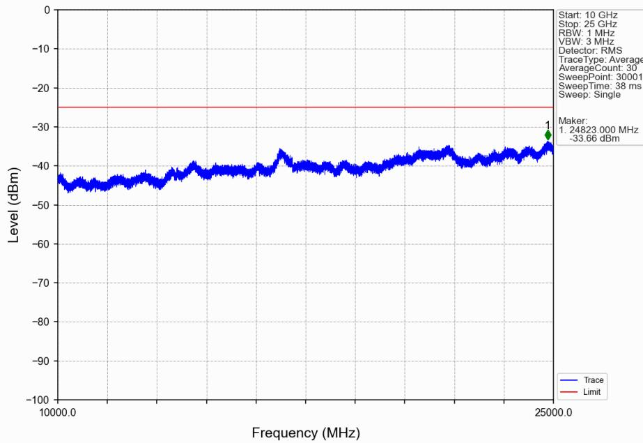
CA\_7C\_SISO\_NTNV\_CC1:10 CC2:20MHz\_CC1:QPSK CC2:QPSK\_CC1:2545.6 CC2:2560MHz\_CC1: 50@0 CC2: 100@0
