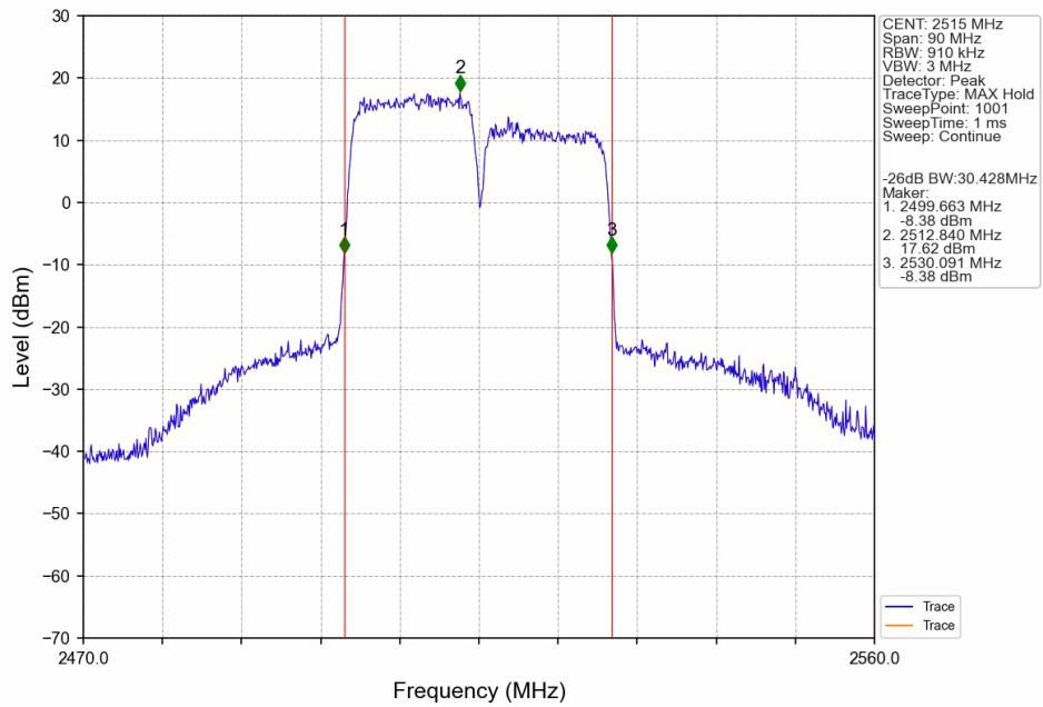
CA\_7C\_SISO\_NTNV\_CC1:15 CC2:15MHz\_CC1:64QAM CC2:64QAM\_CC1:2547.5 CC2:2562.5MHz\_CC1: 75@0 CC2:
