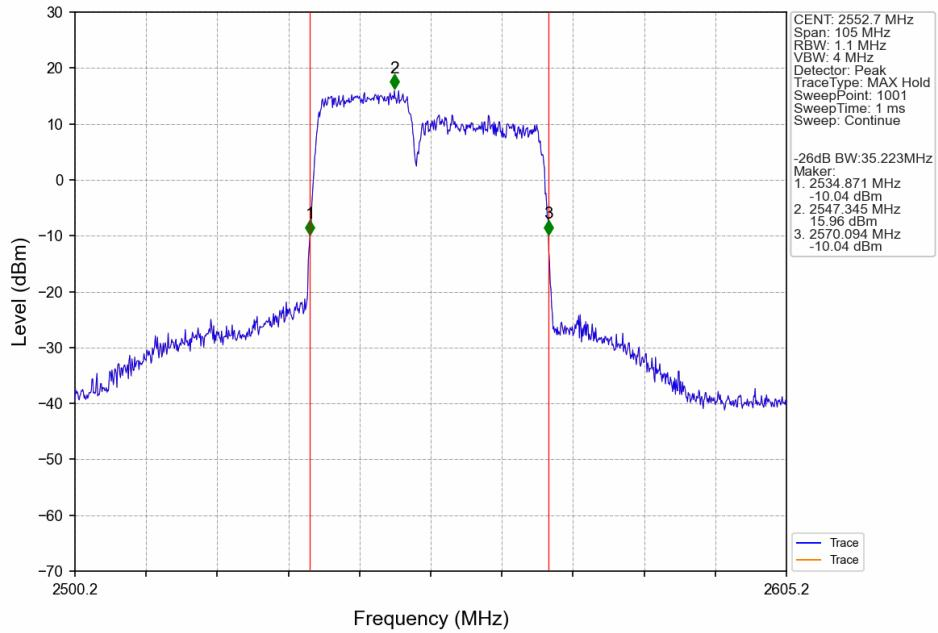
CA\_7C\_SISO\_NTNV\_CC1:20 CC2:10MHz\_CC1:QPSK CC2:QPSK\_CC1:2510 CC2:2524.4MHz\_CC1: 100@0 CC2: 50@0
