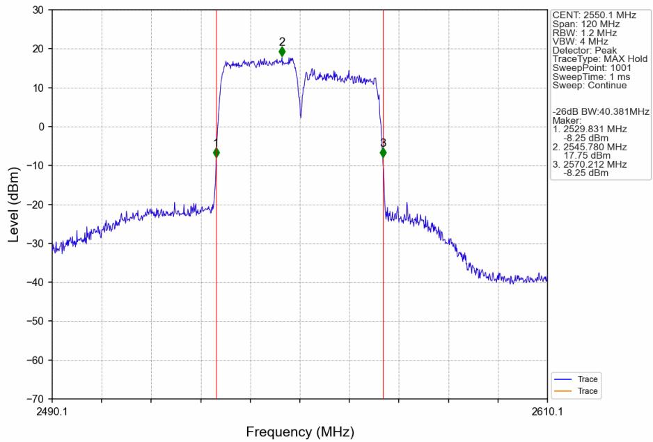
CA\_7C\_SISO\_NTNV\_CC1:20 CC2:20MHz\_CC1:16QAM CC2:16QAM\_CC1:2510 CC2:2529.8MHz\_CC1: 100@0 CC2:
