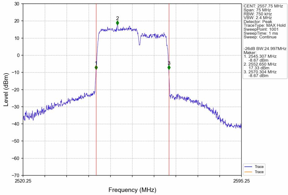
CA\_7C\_SISO\_NTNV\_CC1:15 CC2:10MHz\_CC1:64QAM CC2:64QAM\_CC1:2507.5 CC2:2519.5MHz\_CC1: 75@0 CC2: 50@0
