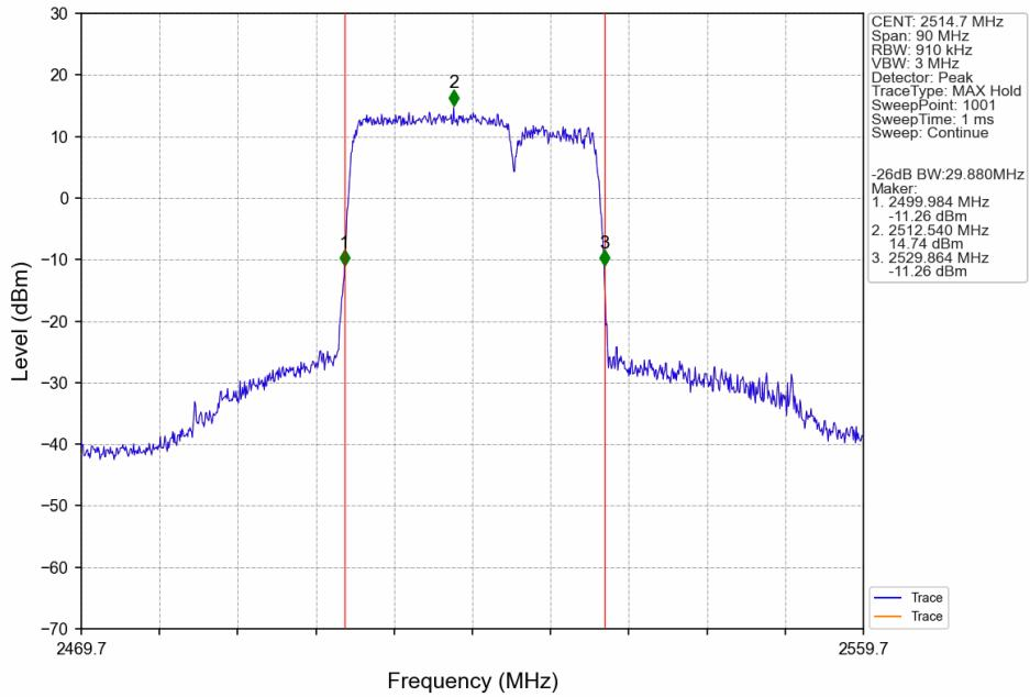
CA\_7C\_SISO\_NTNV\_CC1:20 CC2:10MHz\_CC1:256QAM CC2:256QAM\_CC1:2550.6 CC2:2565MHz\_CC1: 100@0 CC2:
