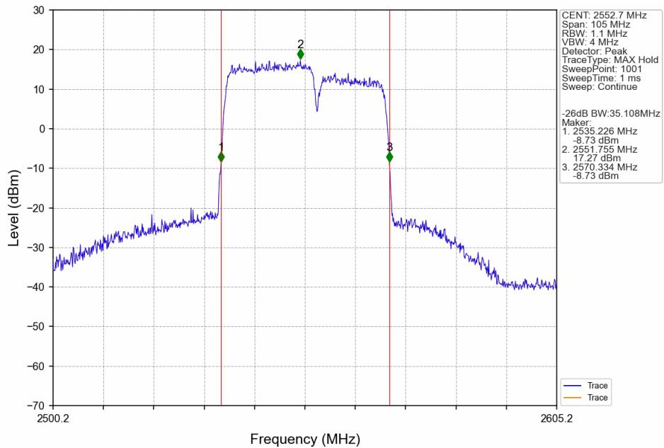
CA\_7C\_SISO\_NTNV\_CC1:20 CC2:15MHz\_CC1:256QAM CC2:256QAM\_CC1:2510 CC2:2527.1MHz\_CC1: 100@0 CC2: 75@0
