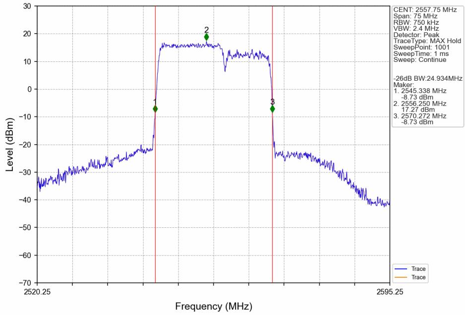
CA\_7C\_SISO\_NTNV\_CC1:15 CC2:10MHz\_CC1:16QAM CC2:16QAM\_CC1:2507.5 CC2:2519.5MHz\_CC1: 75@0 CC2: 50@0
