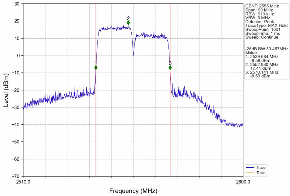
CA\_7C\_SISO\_NTNV\_CC1:15 CC2:15MHz\_CC1:256QAM CC2:256QAM\_CC1:2507.5 CC2:2522.5MHz\_CC1: 75@0 CC2:
