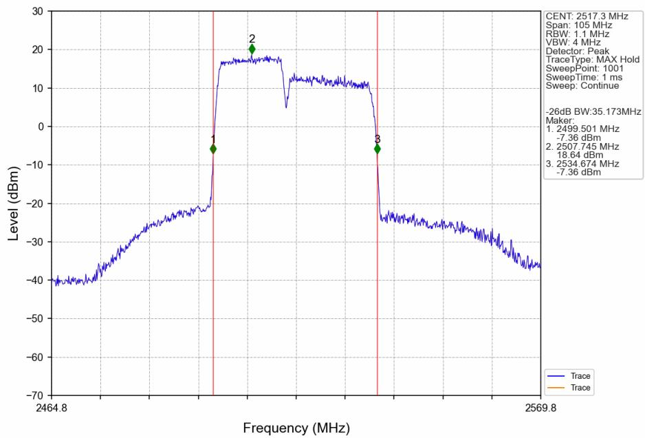
CA\_7C\_SISO\_NTNV\_CC1:15 CC2:20MHz\_CC1:QPSK CC2:QPSK\_CC1:2542.9 CC2:2560MHz\_CC1: 75@0 CC2: 100@0
