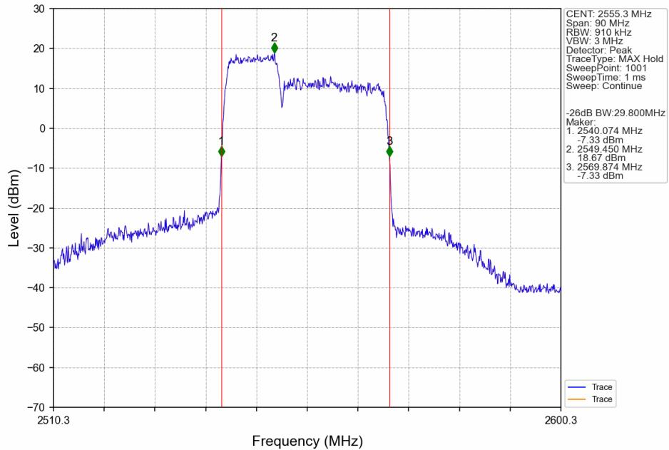
CA\_7C\_SISO\_NTNV\_CC1:10 CC2:20MHz\_CC1:64QAM CC2:64QAM\_CC1:2505 CC2:2519.4MHz\_CC1: 50@0 CC2:
