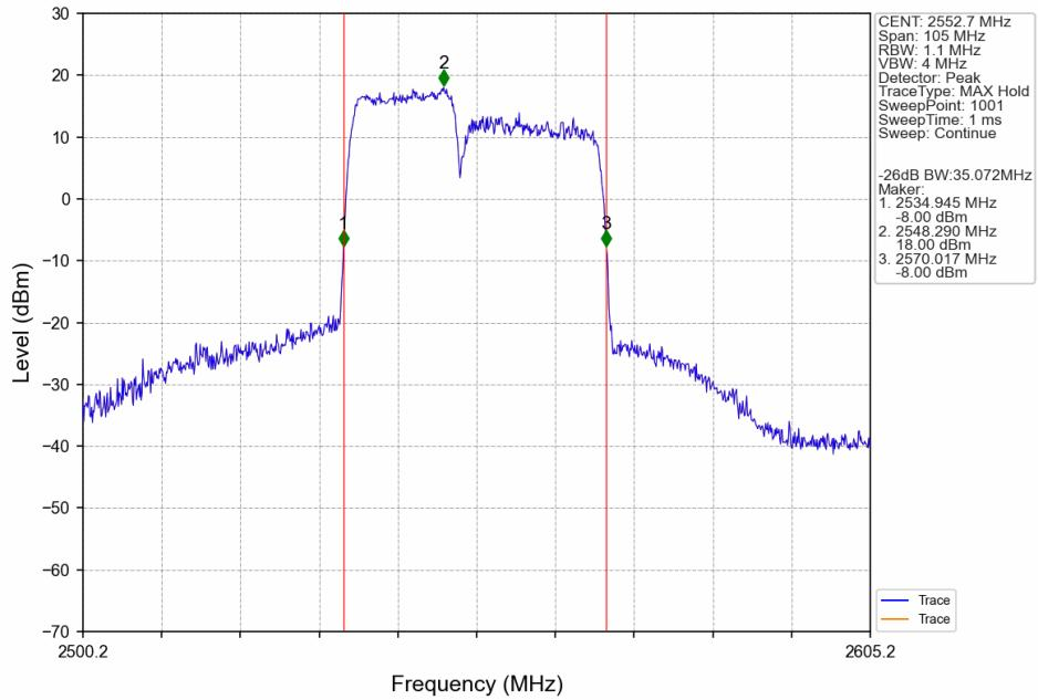
CA\_7C\_SISO\_NTNV\_CC1:15 CC2:20MHz\_CC1:256QAM CC2:256QAM\_CC1:2507.5 CC2:2524.6MHz\_CC1: 75@0 CC2:
