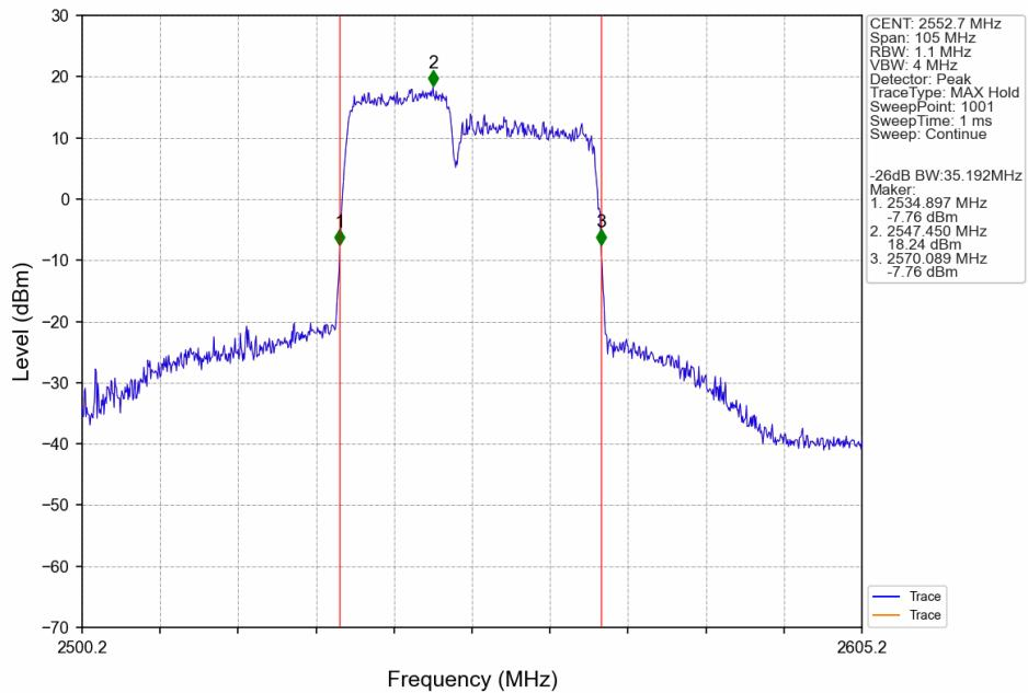
CA\_7C\_SISO\_ntnv\_CC1:15 CC2:20MHz\_CC1:64QAM CC2:64QAM\_CC1:2507.5 CC2:2524.6MHz\_CC1: 75@0 CC2:
