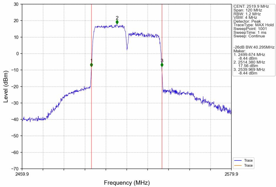
CA\_7C\_SISO\_NTNU\_CC1:20 CC2:20MHz\_CC1:QPSK CC2:QPSK\_CC1:2540.2 CC2:2560MHz\_CC1: 100@0 CC2: 100@0
