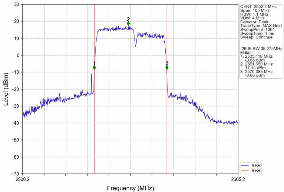
CA\_7C\_SISO\_NTNV\_CC1:20 CC2:15MHz\_CC1:64QAM CC2:64QAM\_CC1:2510 CC2:2527.1MHz\_CC1: 100@0 CC2:
