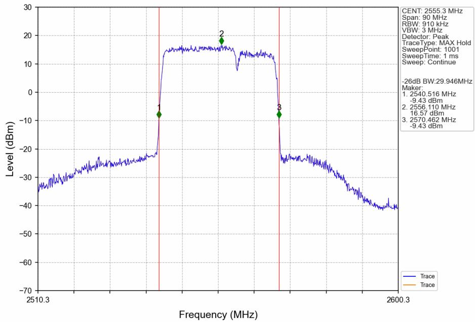
CA\_7C\_SISO\_ntnv\_CC1:20 CC2:10MHz\_CC1:16QAM CC2:16QAM\_CC1:2510 CC2:2524.4MHz\_CC1: 100@0 CC2: 50@0
