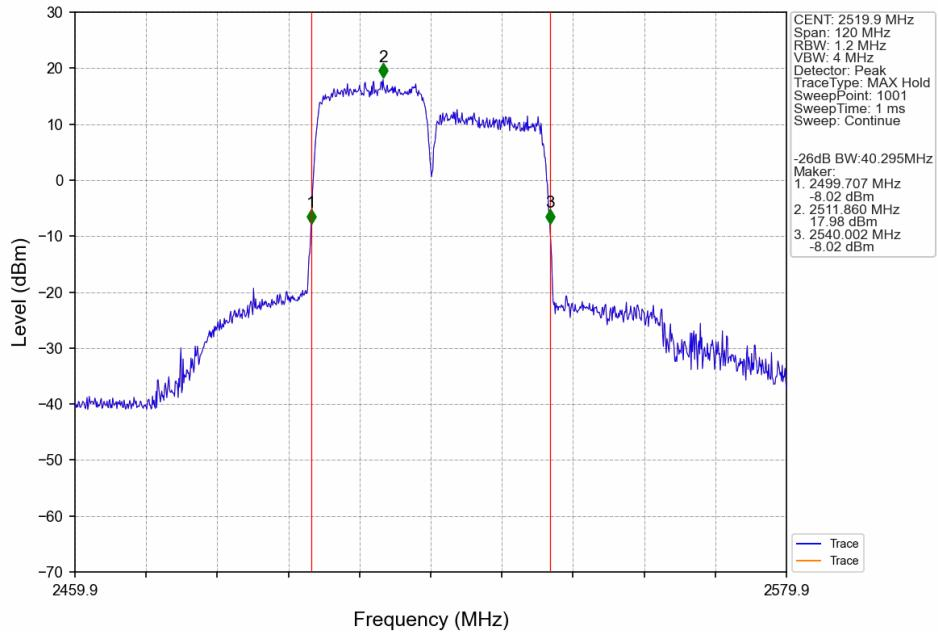
CA\_7C\_SISO\_NTNV\_CC1:20 CC2:20MHz\_CC1:16QAM CC2:16QAM\_CC1:2540.2 CC2:2560MHz\_CC1: 100@0 CC2:
