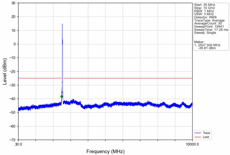
CA\_7C\_SISO\_NTNV\_CC1:10 CC2:20MHz\_CC1:QPSK CC2:QPSK\_CC1:2545.6 CC2:2560MHz\_CC1: 50@0 CC2: 100@0
