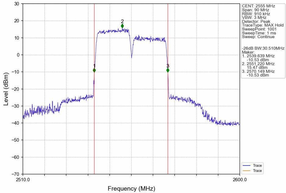
CA\_7C\_SISO\_NTNV\_CC1:15 CC2:20MHz\_CC1:QPSK CC2:QPSK\_CC1:2507.5 CC2:2524.6MHz\_CC1: 75@0 CC2: 100@0
