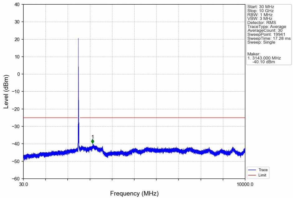
CA\_7C\_SISO\_NTNV\_CC1:10 CC2:20MHz\_CC1:64QAM CC2:64QAM\_CC1:2505 CC2:2519.4MHz\_CC1: 1@0 CC2: 1@0
