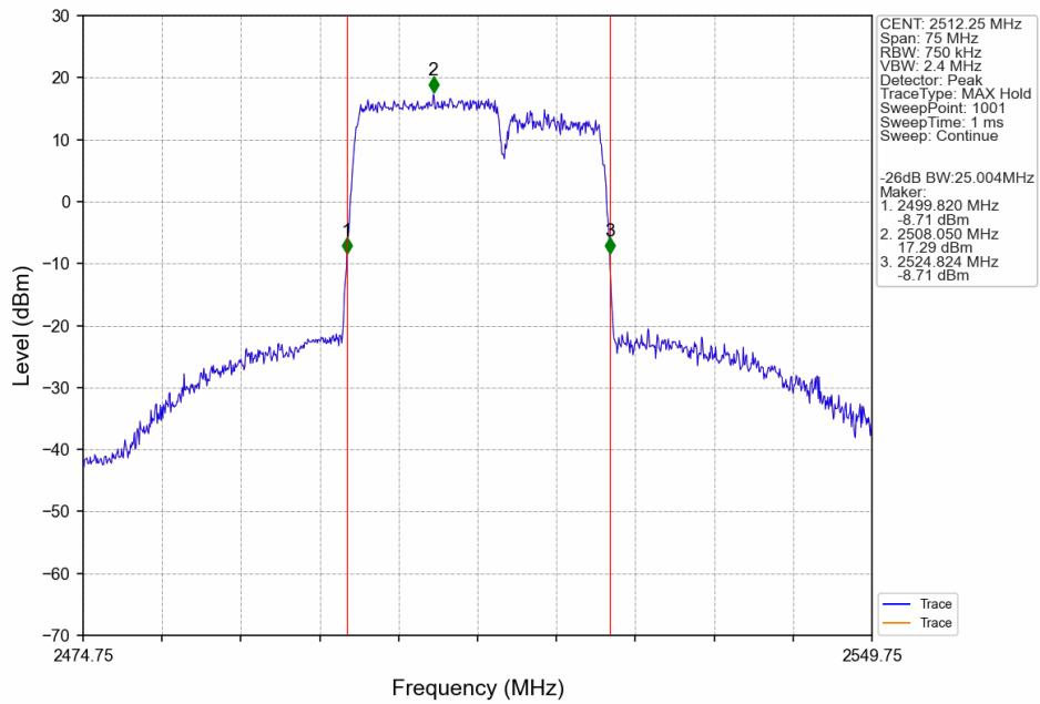
CA\_7C\_SISO\_NTNV\_CC1:15 CC2:10MHz\_CC1:QPSK CC2:QPSK\_CC1:2553 CC2:2565MHz\_CC1: 75@0 CC2: 50@0
