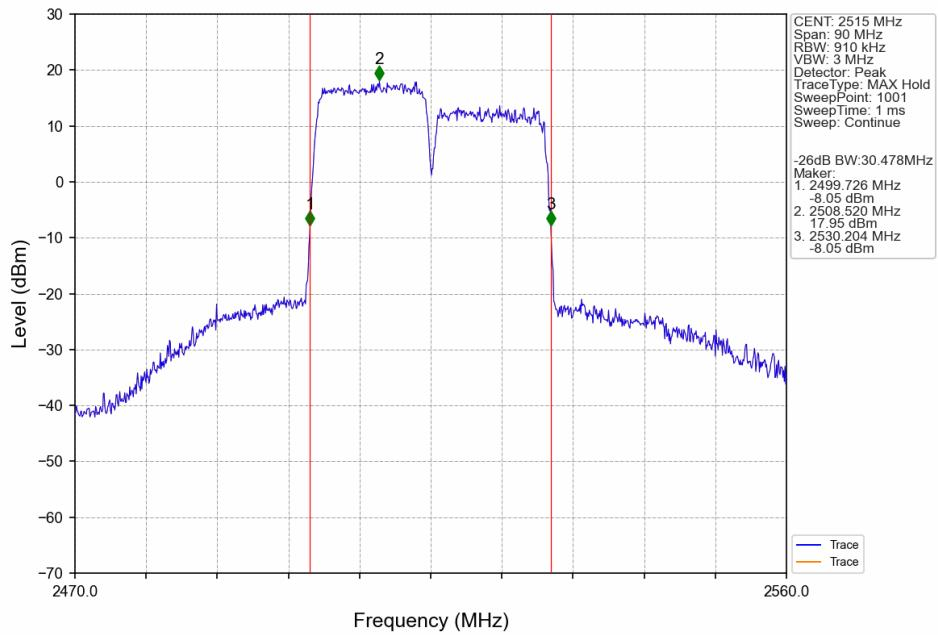
CA\_7C\_SISO\_NTNV\_CC1:15 CC2:15MHz\_CC1:QPSK CC2:QPSK\_CC1:2547.5 CC2:2562.5MHz\_CC1: 75@0 CC2: 75@0
