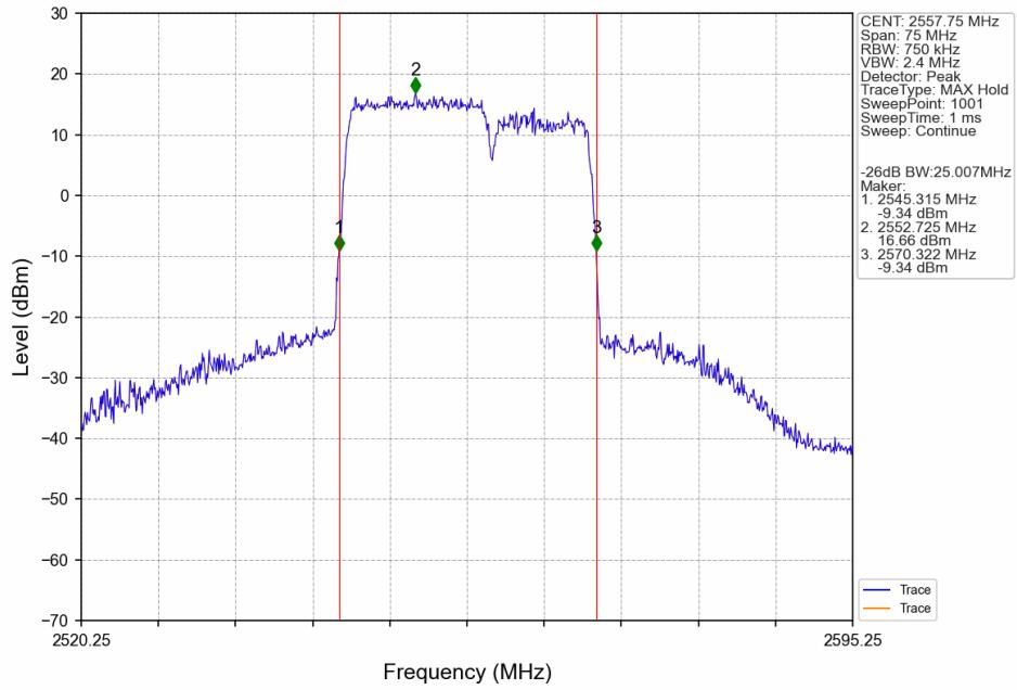
CA\_7C\_SISO\_NTNV\_CC1:15 CC2:10MHz\_CC1:256QAM CC2:256QAM\_CC1:2507.5 CC2:2519.5MHz\_CC1: 75@0 CC2: 50@0
