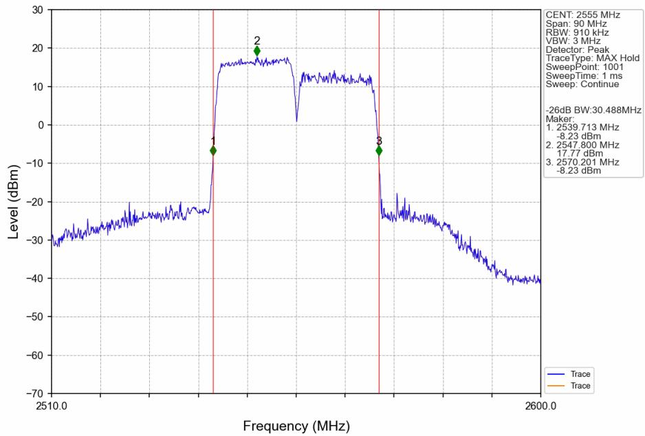
CA\_7C\_SISO\_NTNV\_CC1:15 CC2:15MHz\_CC1:16QAM CC2:16QAM\_CC1:2507.5 CC2:2522.5MHz\_CC1: 75@0 CC2: 75@0
