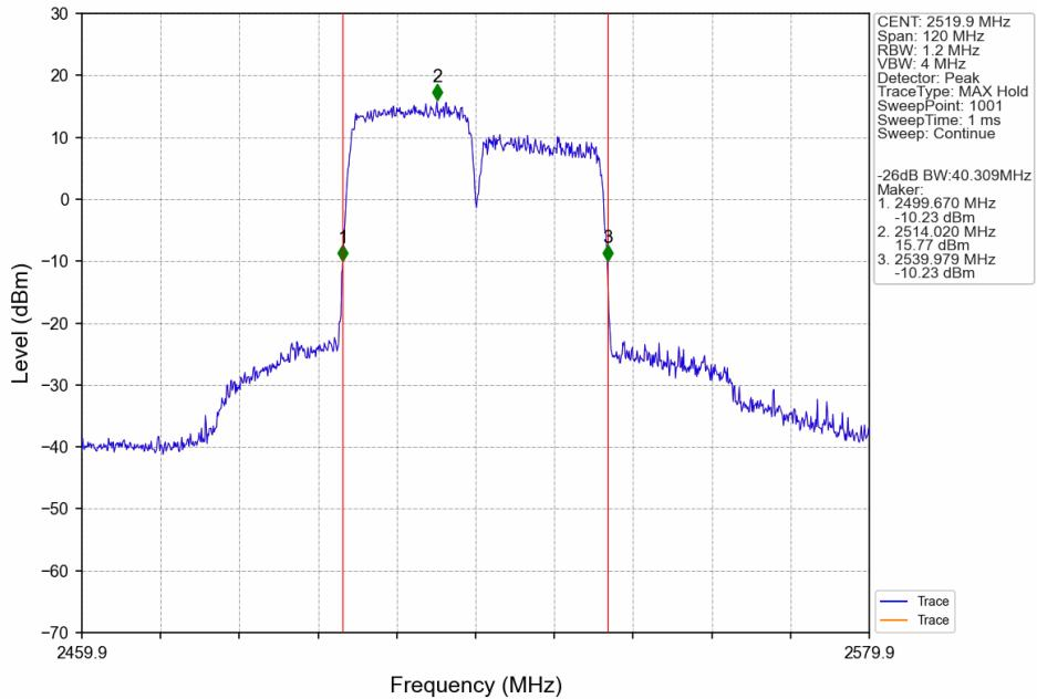
CA\_7C\_SISO\_NTNV\_CC1:20 CC2:20MHz\_CC1:256QAM CC2:256QAM\_CC1:2540.2 CC2:2560MHz\_CC1: 100@0 CC2:
