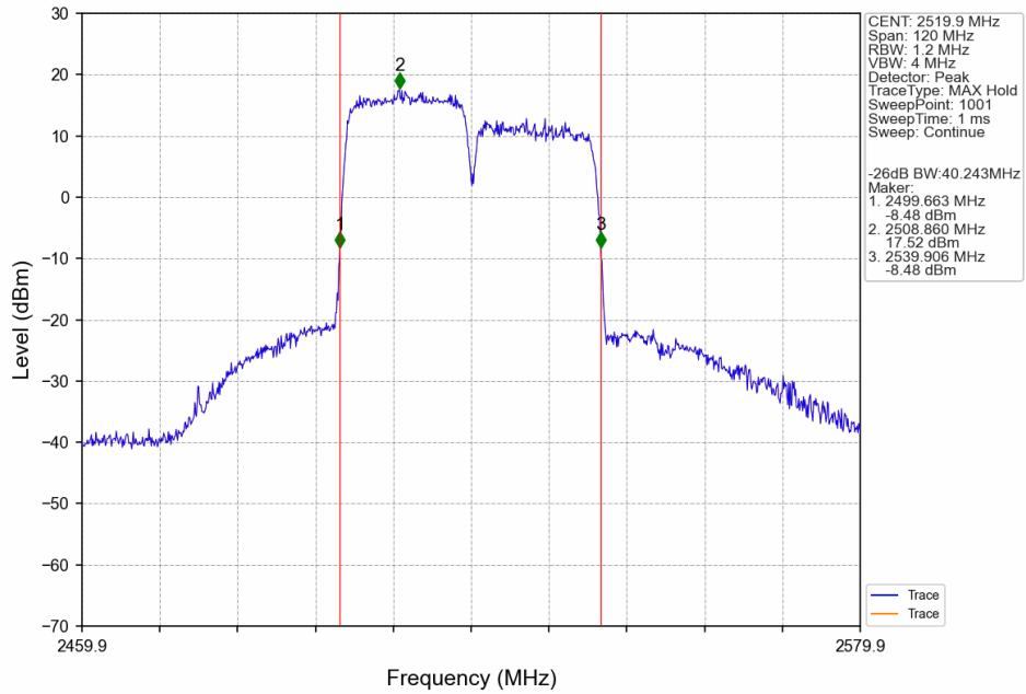
CA\_7C\_SISO\_NTNV\_CC1:20 CC2:20MHz\_CC1:64QAM CC2:64QAM\_CC1:2540.2 CC2:2560MHz\_CC1: 100@0 CC2:
