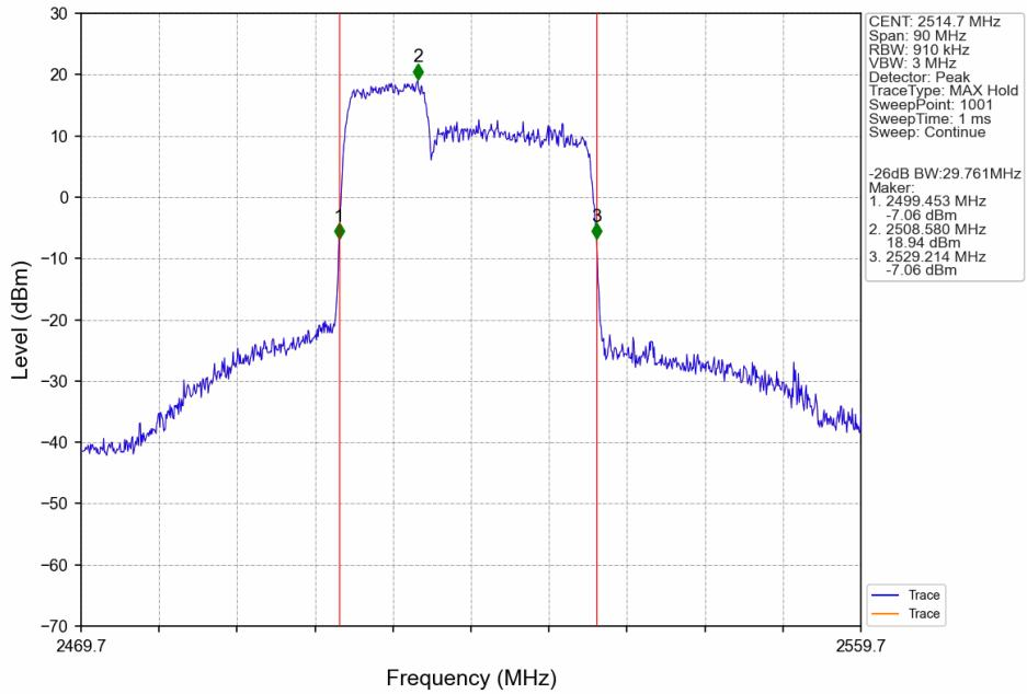
CA\_7C\_SISO\_NTNV\_CC1:10 CC2:20MHz\_CC1:64QAM CC2:64QAM\_CC1:2545.6 CC2:2560MHz\_CC1: 50@0 CC2:
