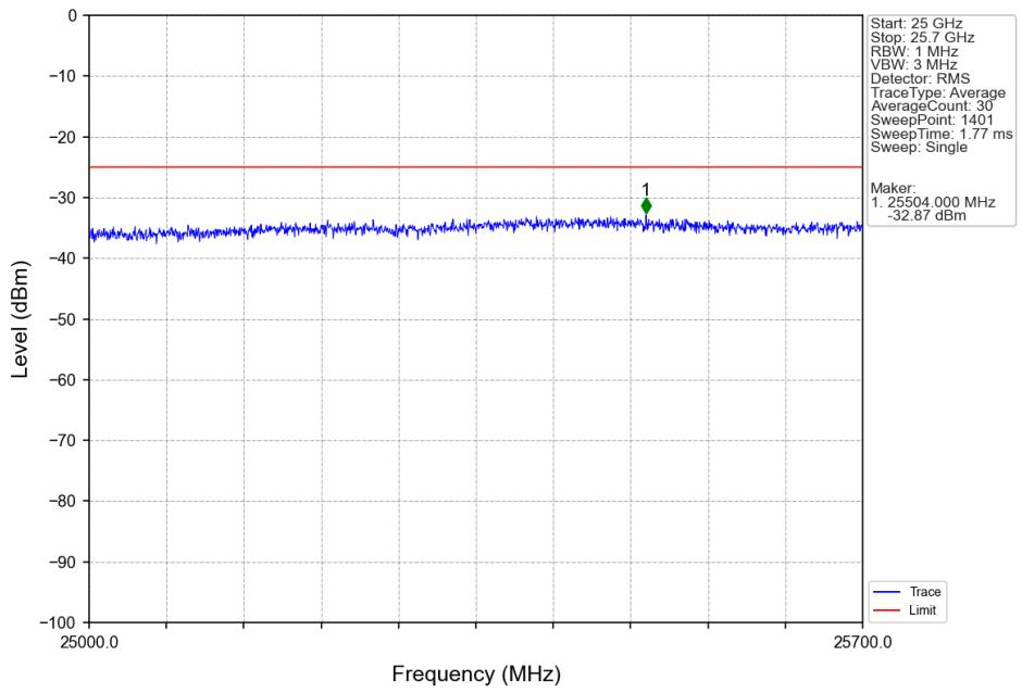
CA\_7C\_SISO\_NTNV\_CC1:10 CC2:20MHz\_CC1:QPSK CC2:QPSK\_CC1:2505 CC2:2519.4MHz\_CC1: 50@0 CC2: 100@0
