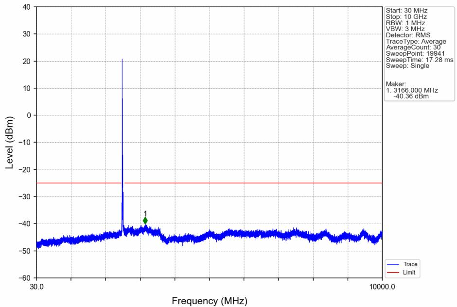
CA\_7C\_SISO\_NTNV\_CC1:10 CC2:20MHz\_CC1:16QAM CC2:16QAM\_CC1:2505 CC2:2519.4MHz\_CC1: 1@0 CC2: 1@0
