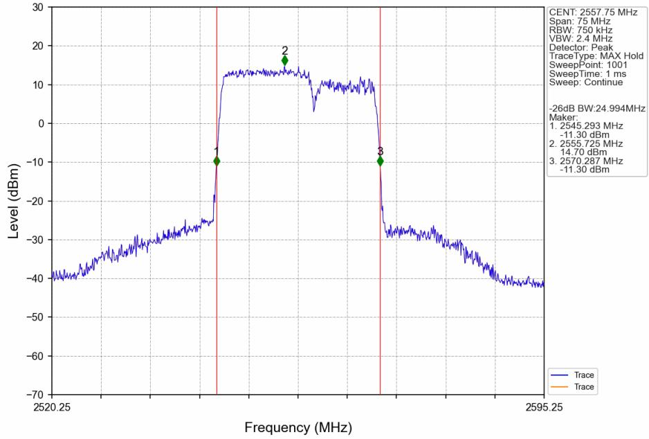
CA\_7C\_SISO\_NTNV\_CC1:15 CC2:15MHz\_CC1:QPSK CC2:QPSK\_CC1:2507.5 CC2:2522.5MHz\_CC1: 75@0 CC2: 75@0
