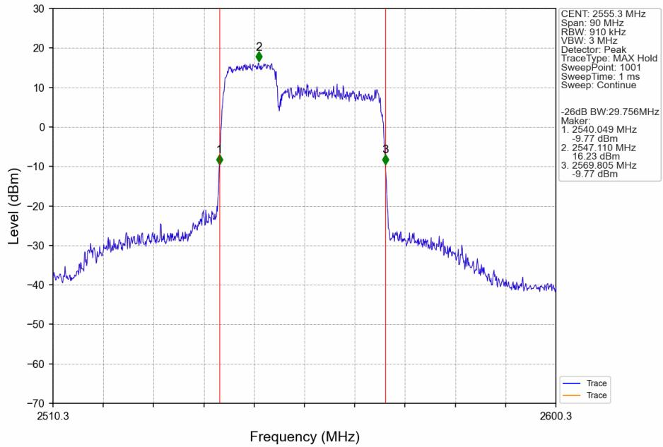
CA\_7C\_SISO\_NTNV\_CC1:15 CC2:10MHz\_CC1:QPSK CC2:QPSK\_CC1:2507.5 CC2:2519.5MHz\_CC1: 75@0 CC2: 50@0
