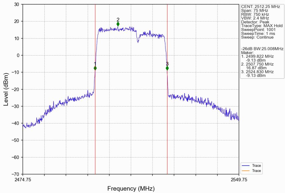
CA\_7C\_SISO\_NTNV\_CC1:15 CC2:10MHz\_CC1:64QAM CC2:64QAM\_CC1:2553 CC2:2565MHz\_CC1: 75@0 CC2: 50@0
