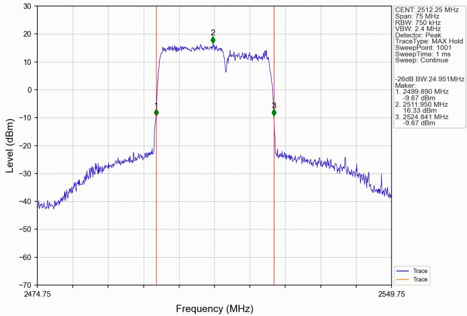
CA\_7C\_SISO\_NTNV\_CC1:15 CC2:10MHz\_CC1:16QAM CC2:16QAM\_CC1:2553 CC2:2565MHz\_CC1: 75@0 CC2: 50@0
