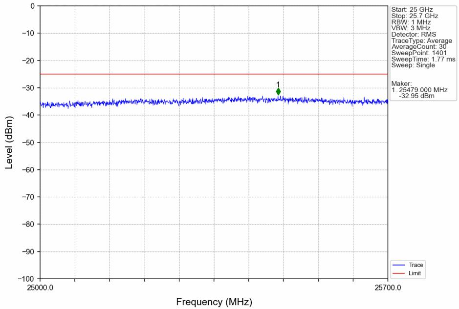
CA\_7C\_SISO\_NTNV\_CC1:10 CC2:20MHz\_CC1:16QAM CC2:16QAM\_CC1:2545.6 CC2:2560MHz\_CC1: 1@0 CC2: 1@0
