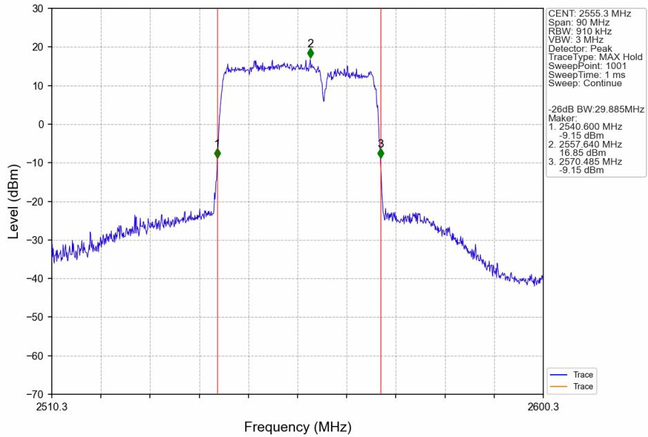
CA\_7C\_SISO\_NTNV\_CC1:20 CC2:10MHz\_CC1:256QAM CC2:256QAM\_CC1:2510 CC2:2524.4MHz\_CC1: 100@0 CC2:
