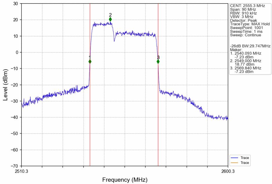
CA\_7C\_SISO\_NTNV\_CC1:10 CC2:20MHz\_CC1:256QAM CC2:256QAM\_CC1:2505 CC2:2519.4MHz\_CC1: 50@0 CC2:
