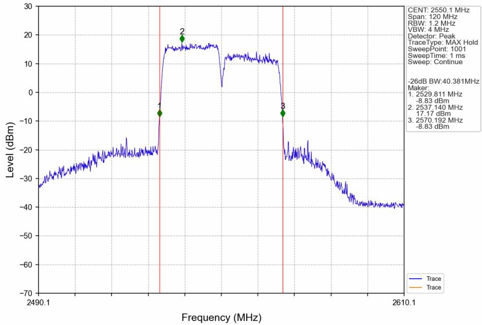
CA\_7C\_SISO\_NTNV\_CC1:20 CC2:20MHz\_CC1:256QAM CC2:256QAM\_CC1:2510 CC2:2529.8MHz\_CC1: 100@0 CC2:
