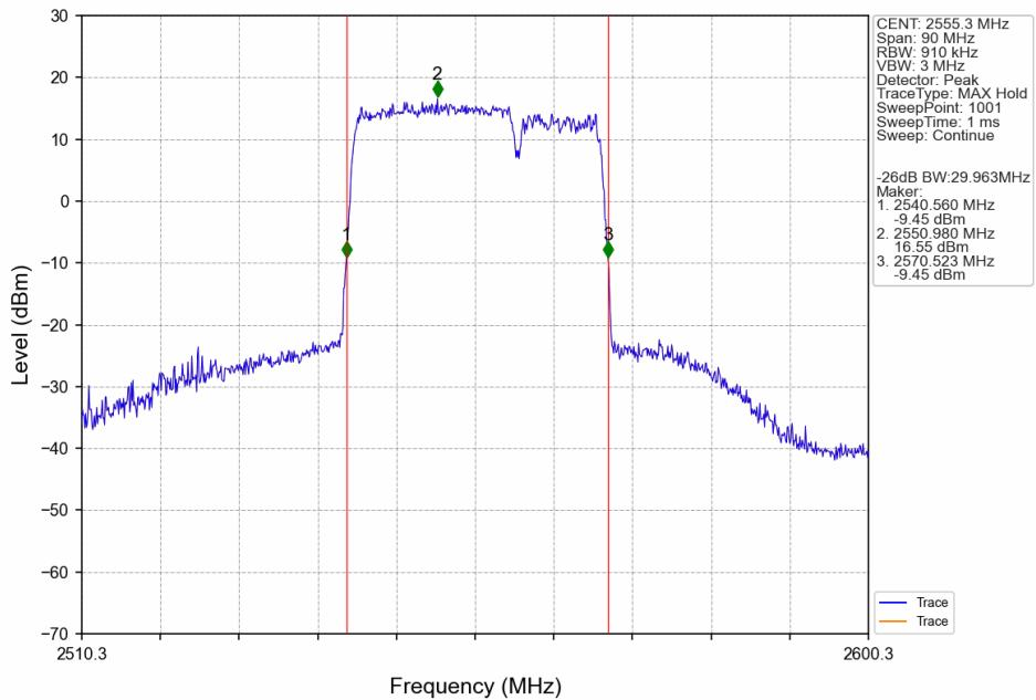
CA\_7C\_SISO\_NTNV\_CC1:20 CC2:10MHz\_CC1:64QAM CC2:64QAM\_CC1:2510 CC2:2524.4MHz\_CC1: 100@0 CC2:
