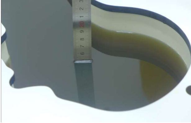
Photo 1: Tissue Simulant Liquid for HBBL600-10000MHz
