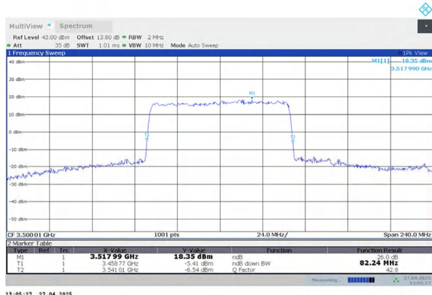
**n78L,80MHz Bandwidth,DFT-s-16QAM (-26dBc BW)**
