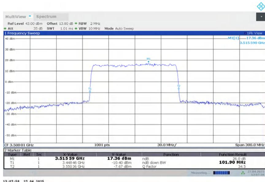
**n78L,100MHz Bandwidth,DFT-s-16QAM (-26dBc BW)**
