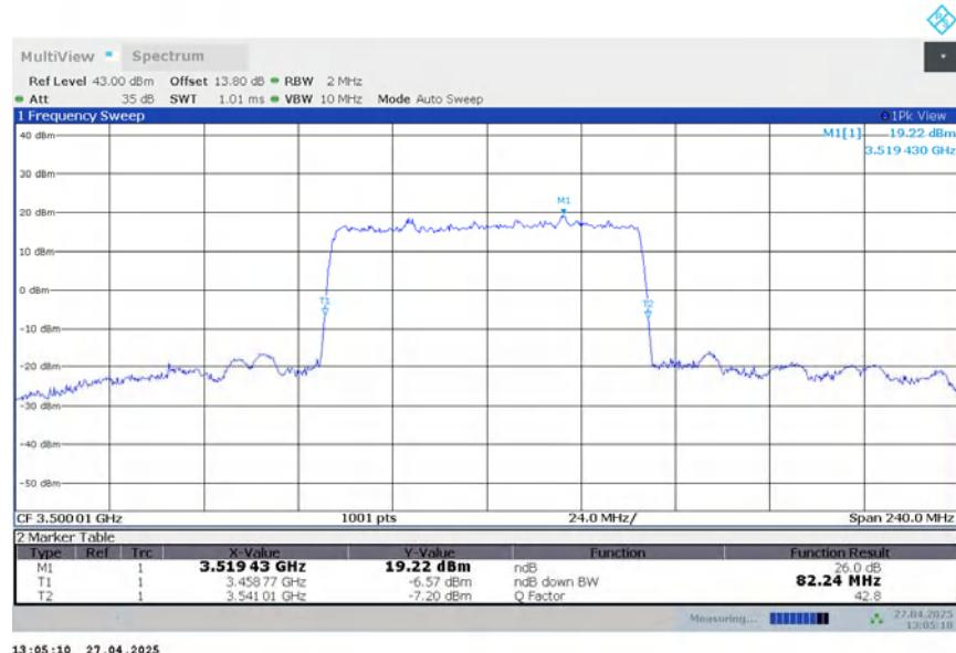
**n78L,80MHz Bandwidth,DFT-s-QPSK (-26dBc BW)**
