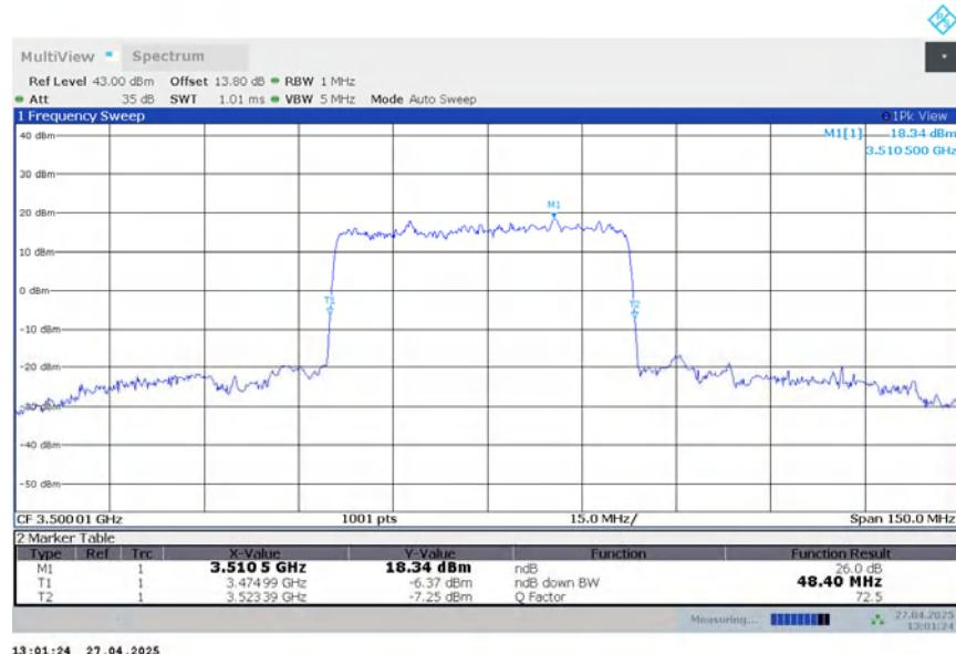
**n78L,50MHz Bandwidth,DFT-s-QPSK (-26dBc BW)**
