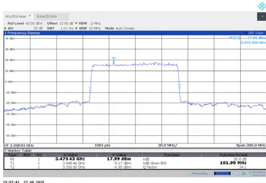
**n78L,100MHz Bandwidth,DFT-s-QPSK (-26dBc BW)**
