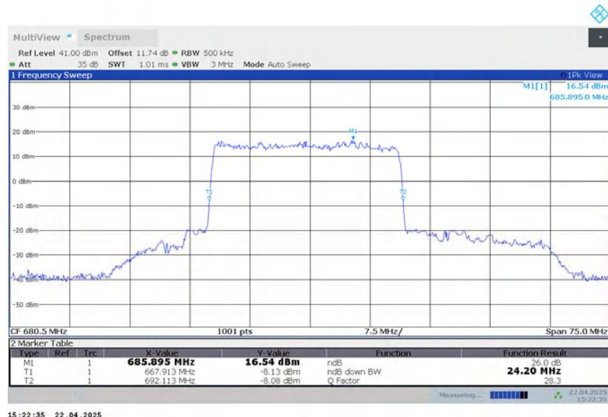
**n71,25MHz Bandwidth,DFT-s-QPSK (-26dBc BW)**
