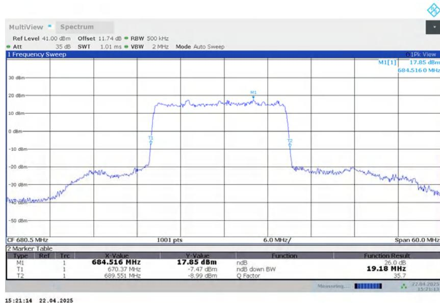
**n71,20MHz Bandwidth,DFT-s-QPSK (-26dBc BW)**
