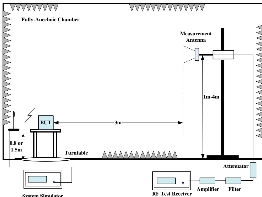
1. The EUT is then put into continuously transmitting mode at its maximum power level during the test. And the maximum value of the receiver should be recorded as (Pr).
