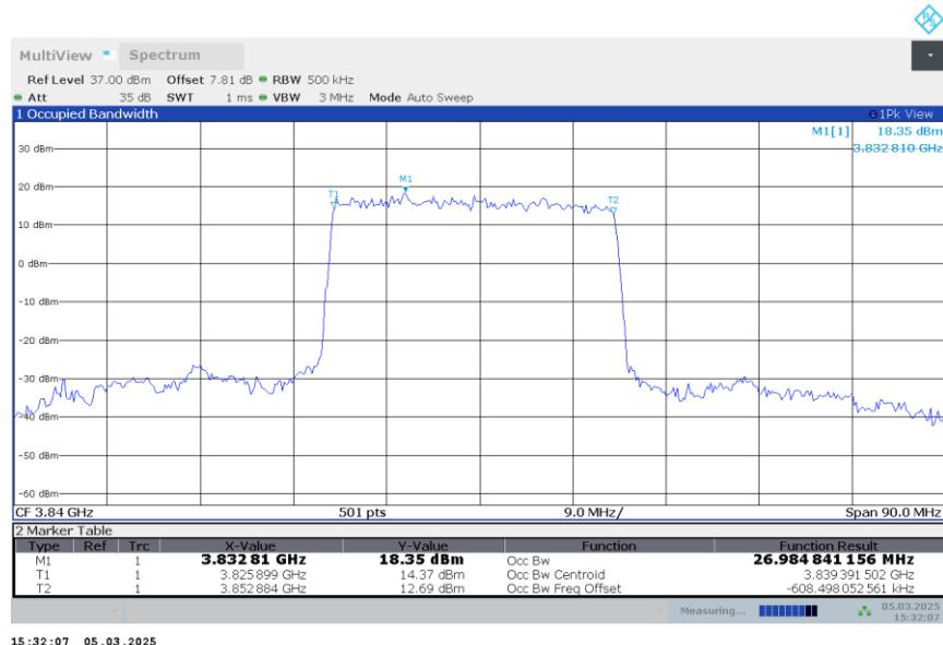
**n77H,30MHz Bandwidth,DFT-s-QPSK (99% BW)**
