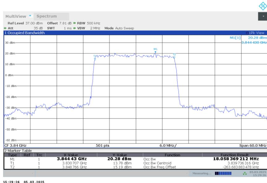
**n77H,20MHz Bandwidth,DFT-s-QPSK (99% BW)**
