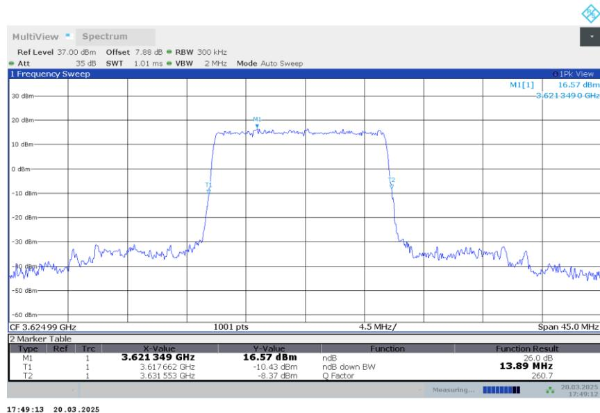
n48,15MHz Bandwidth,DFT-s-QPSK (-26dBc BW)
