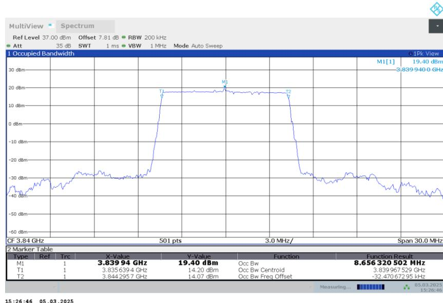
**n77H,10MHz Bandwidth,DFT-s-QPSK (99% BW)**
