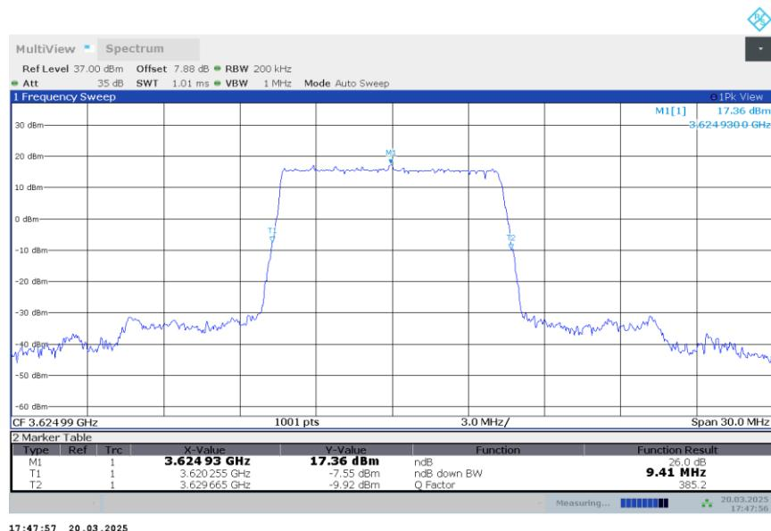
n48,10MHz Bandwidth,DFT-s-QPSK (-26dBc BW)
