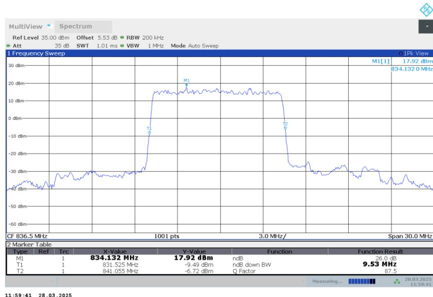
n5,10MHz Bandwidth,DFT-s-QPSK (-26dBc BW)
