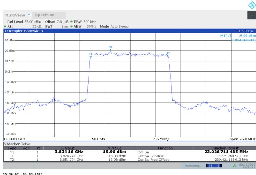
**n77H,25MHz Bandwidth,DFT-s-QPSK (99% BW)**
