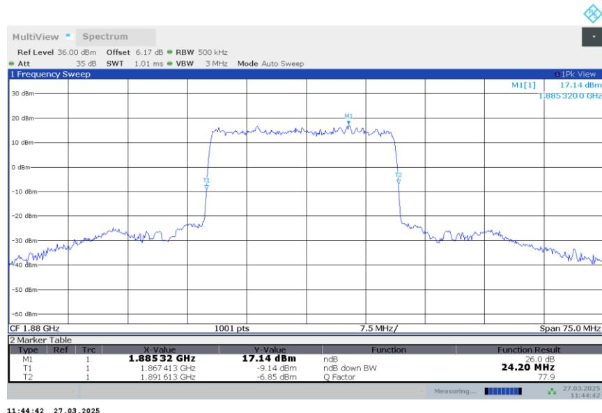
n2,25MHz Bandwidth,DFT-s-QPSK (-26dBc BW)
