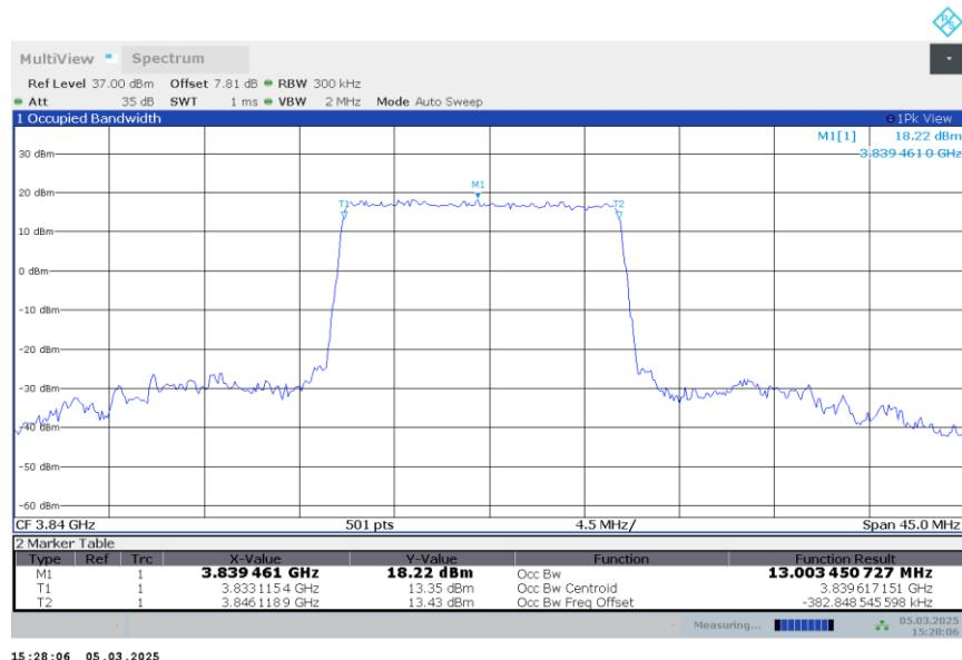
**n77H,15MHz Bandwidth,DFT-s-QPSK (99% BW)**
