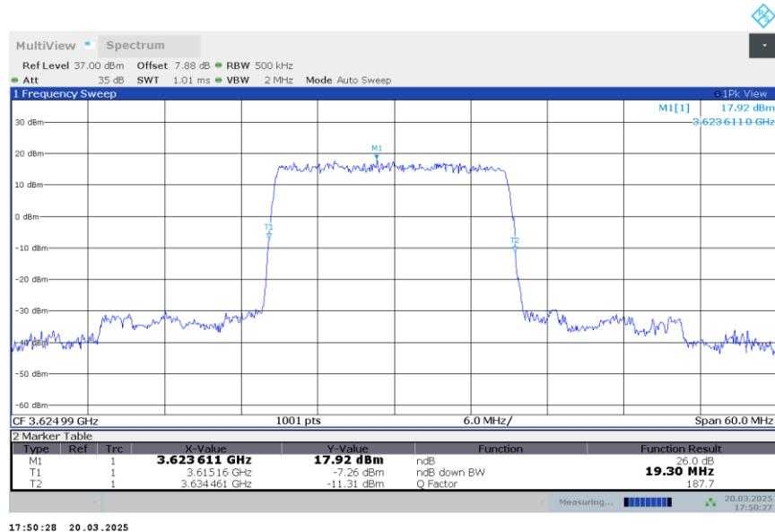
n48,20MHz Bandwidth,DFT-s-QPSK (-26dBc BW)
