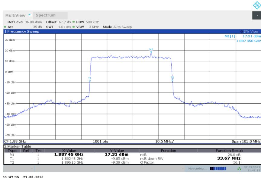
n2,35MHz Bandwidth,DFT-s-QPSK (-26dBc BW)
