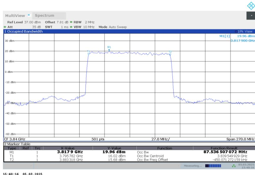
**n77H,90MHz Bandwidth,DFT-s-QPSK (99% BW)**
