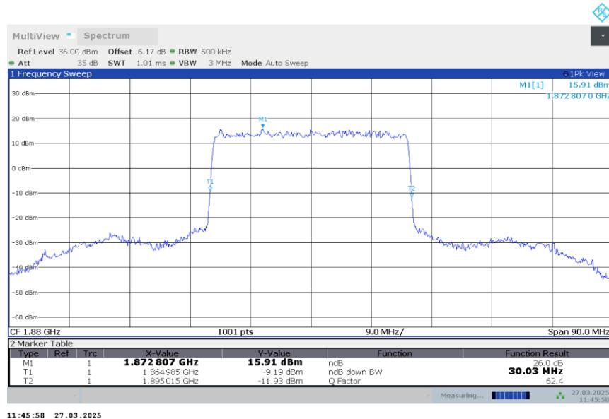
n2,30MHz Bandwidth,DFT-s-QPSK (-26dBc BW)
