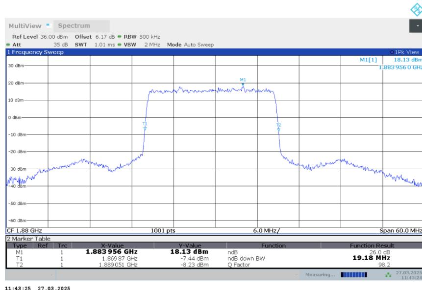
**n2,20MHz Bandwidth,DFT-s-QPSK (-26dBc BW)**
