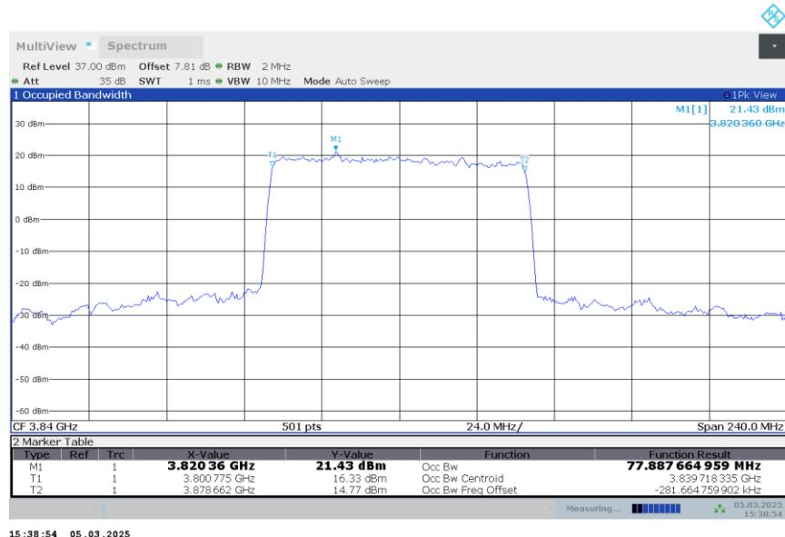
**n77H,80MHz Bandwidth,DFT-s-QPSK (99% BW)**
