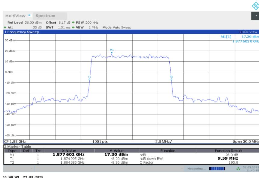
n2,10MHz Bandwidth,DFT-s-QPSK (-26dBc BW)
