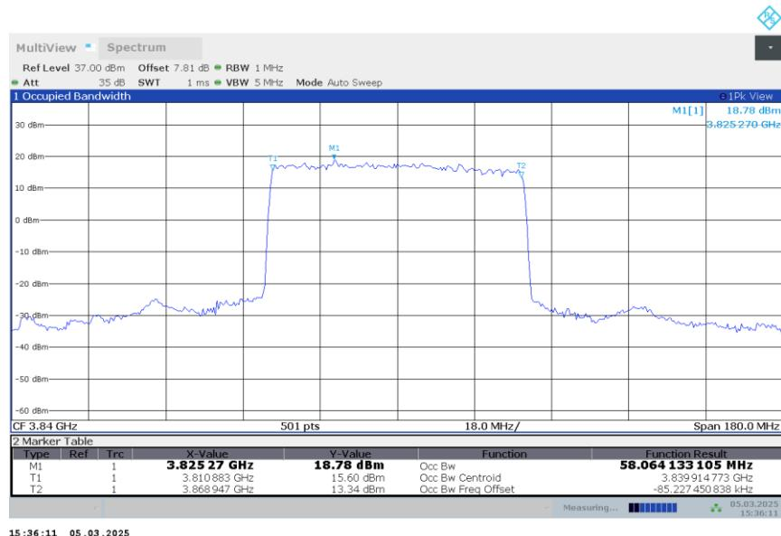
**n77H,60MHz Bandwidth,DFT-s-QPSK (99% BW)**
