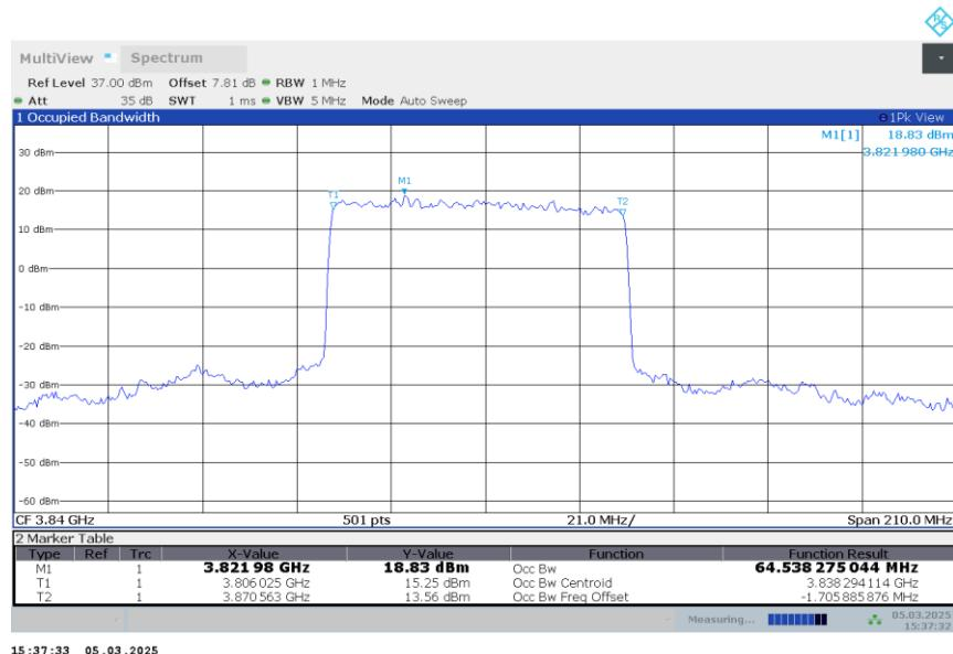
**n77H,70MHz Bandwidth,DFT-s-QPSK (99% BW)**
