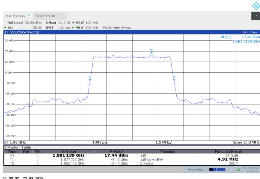
n2,5MHz Bandwidth,DFT-s-QPSK (-26dBc BW)
