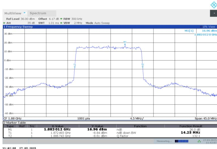
n2,15MHz Bandwidth,DFT-s-QPSK (-26dBc BW)
