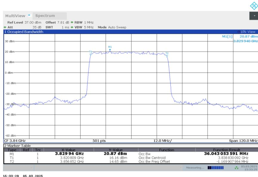
**n77H,40MHz Bandwidth,DFT-s-QPSK (99% BW)**
