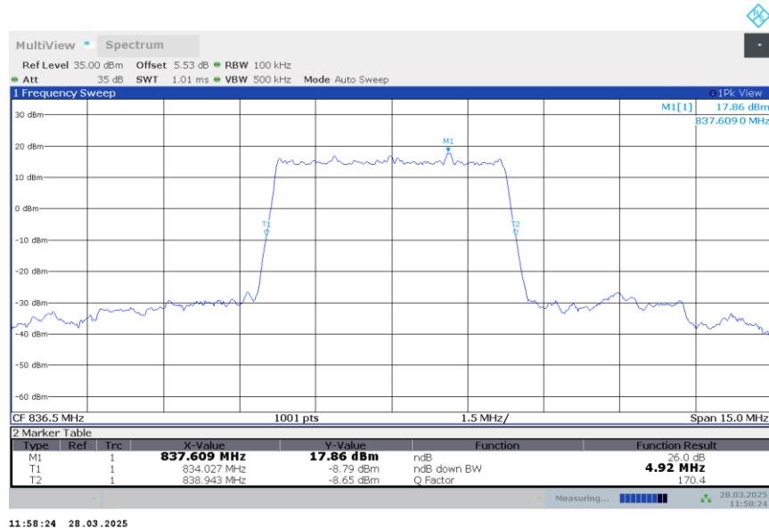
n5,5MHz Bandwidth,DFT-s-QPSK (-26dBc BW)
