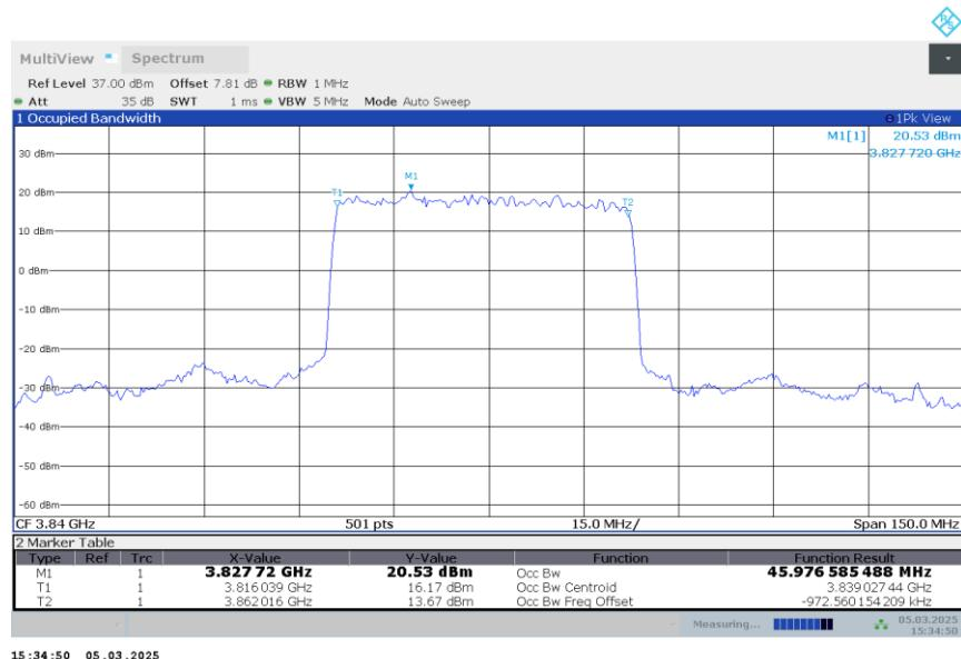
**n77H,50MHz Bandwidth,DFT-s-QPSK (99% BW)**
