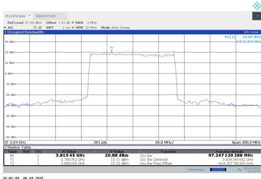
**n77H,100MHz Bandwidth,DFT-s-QPSK (99% BW)**
