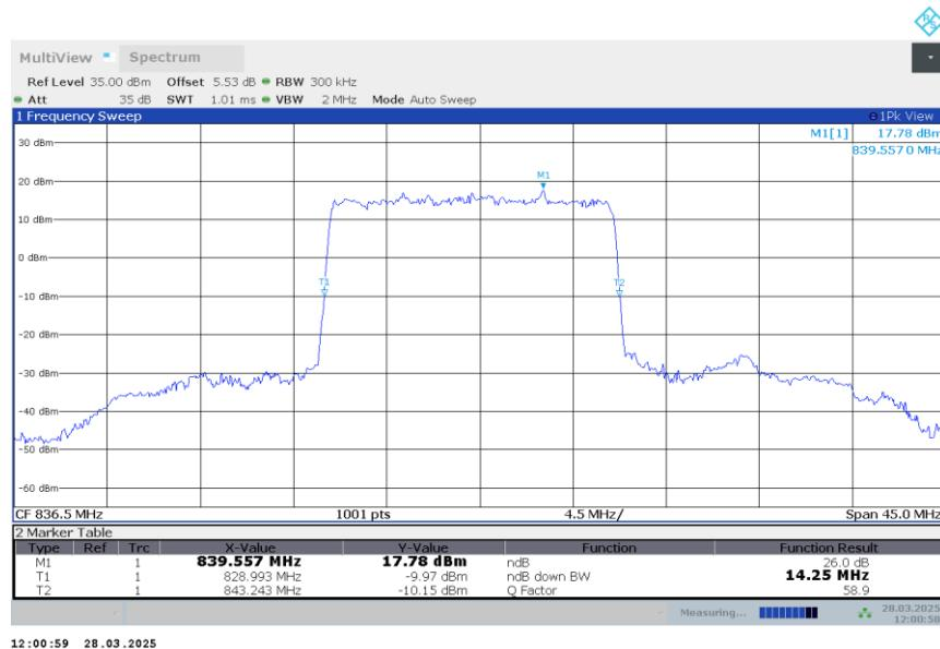
n5,15MHz Bandwidth,DFT-s-QPSK (-26dBc BW)
