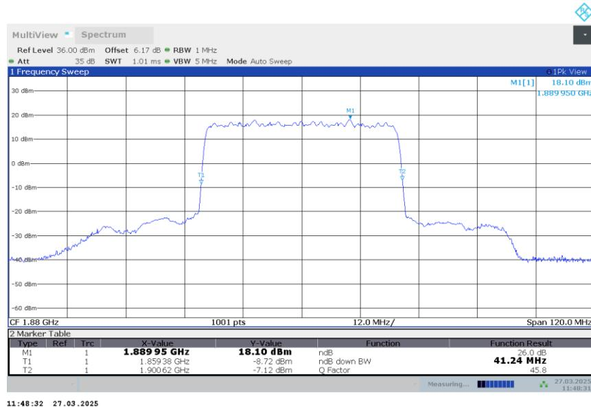
**n2,40MHz Bandwidth,DFT-s-QPSK (-26dBc BW)**
