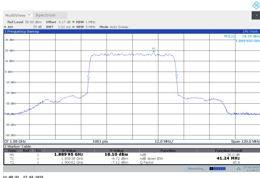
**n2,40MHz Bandwidth,DFT-s-QPSK (-26dBc BW)**
