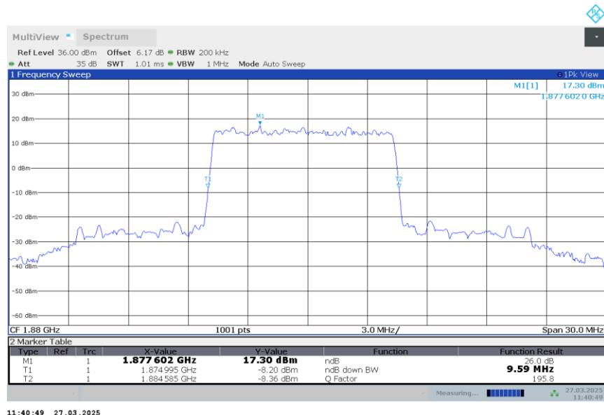
n2,10MHz Bandwidth,DFT-s-QPSK (-26dBc BW)
