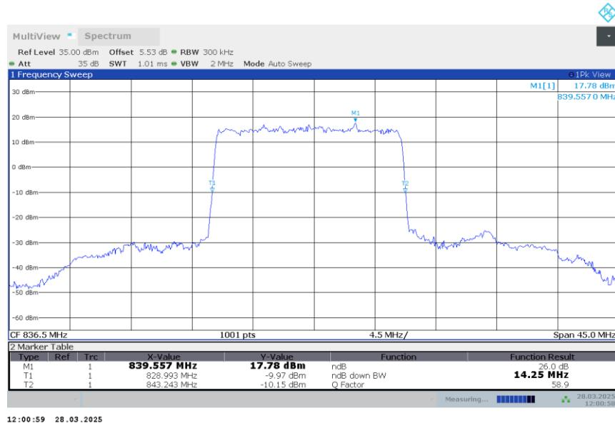
n5,15MHz Bandwidth,DFT-s-QPSK (-26dBc BW)
