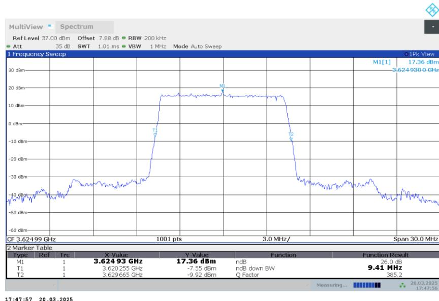
**n48,10MHz Bandwidth,DFT-s-QPSK (-26dBc BW)**
