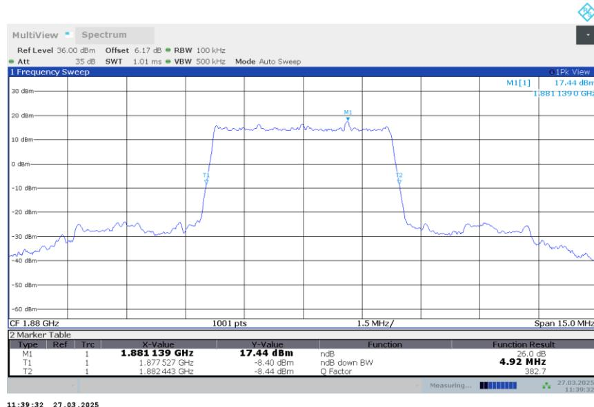
n2,5MHz Bandwidth,DFT-s-QPSK (-26dBc BW)
