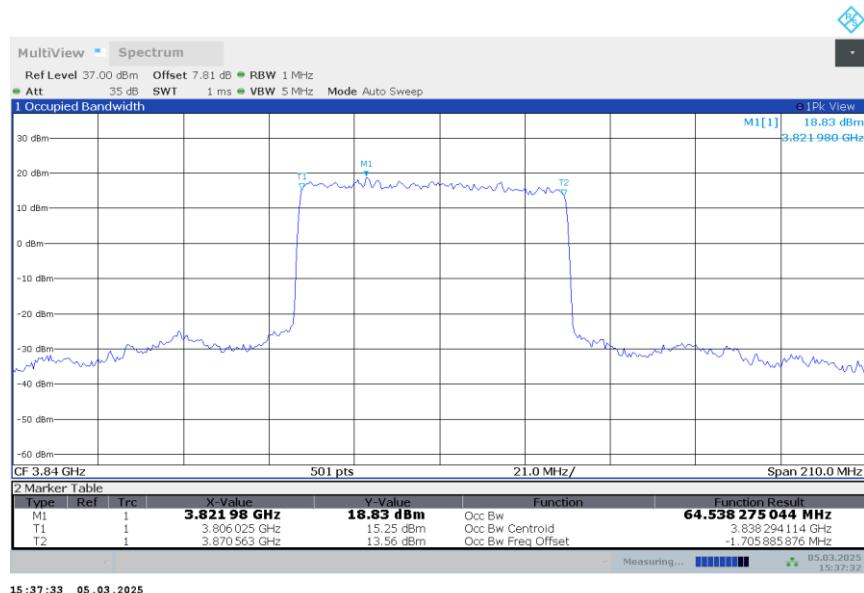
**n77H,70MHz Bandwidth,DFT-s-QPSK (99% BW)**
