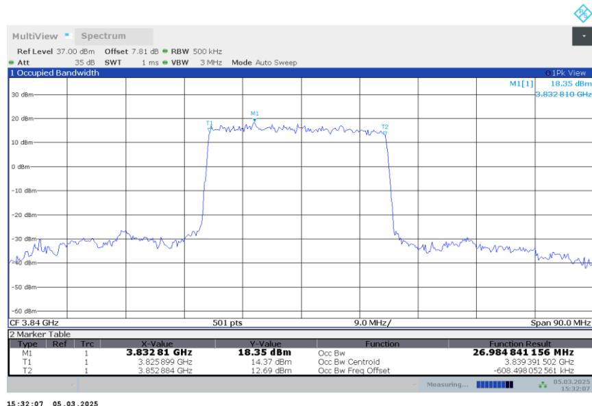
**n77H,30MHz Bandwidth,DFT-s-QPSK (99% BW)**
