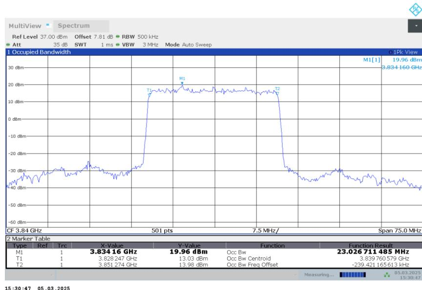
**n77H,25MHz Bandwidth,DFT-s-QPSK (99% BW)**
