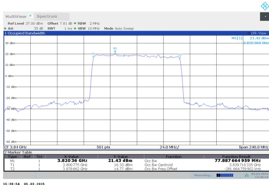
**n77H,80MHz Bandwidth,DFT-s-QPSK (99% BW)**
