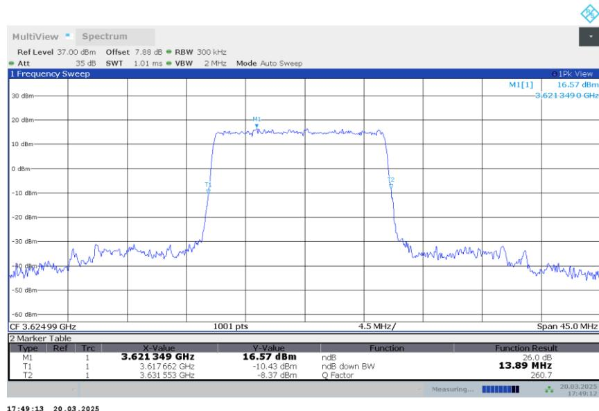
n48,15MHz Bandwidth,DFT-s-QPSK (-26dBc BW)
