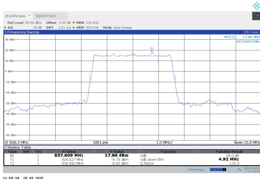
n5,5MHz Bandwidth,DFT-s-QPSK (-26dBc BW)
