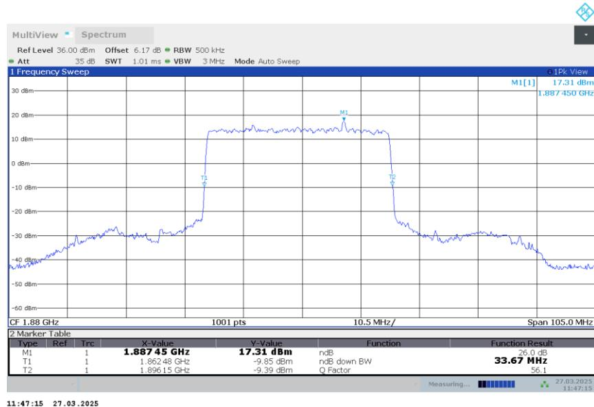
n2,35MHz Bandwidth,DFT-s-QPSK (-26dBc BW)
