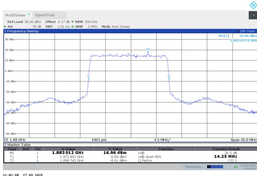
n2,15MHz Bandwidth,DFT-s-QPSK (-26dBc BW)
