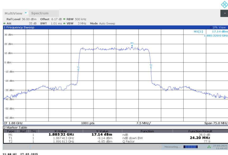
n2,25MHz Bandwidth,DFT-s-QPSK (-26dBc BW)
