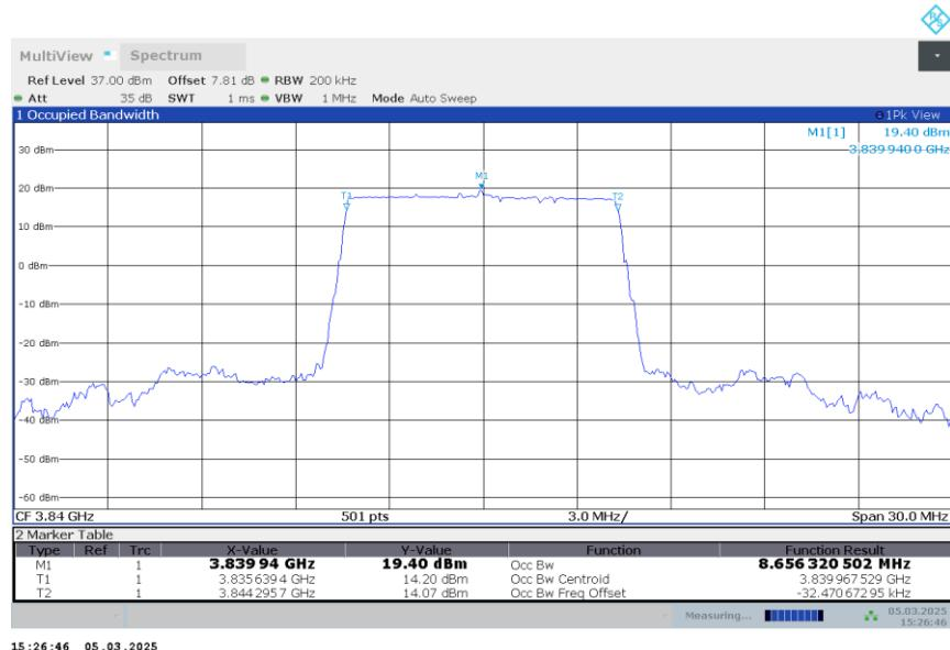
**n77H,10MHz Bandwidth,DFT-s-QPSK (99% BW)**
