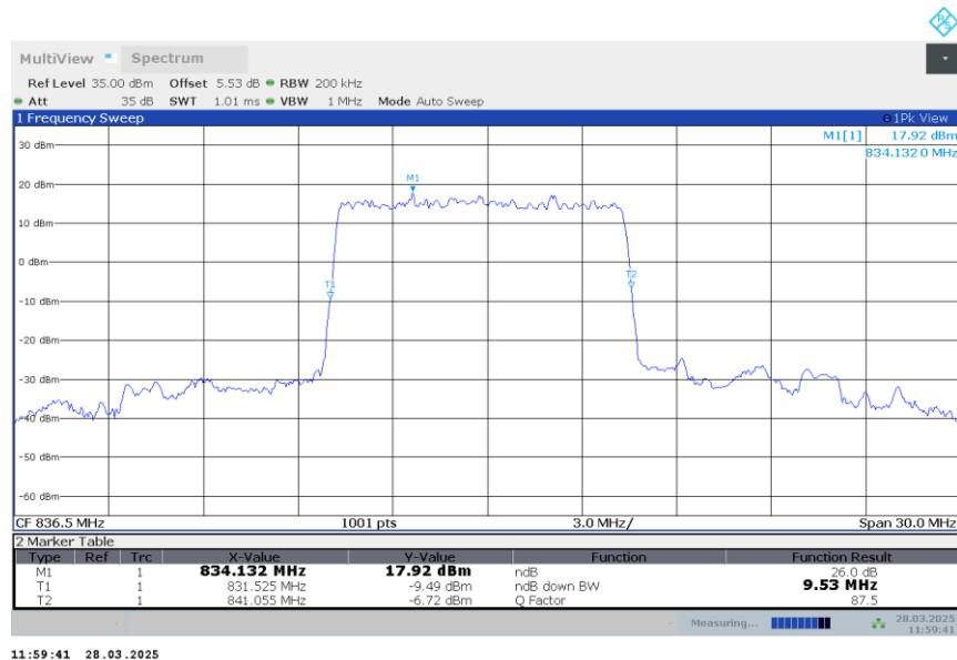
n5,10MHz Bandwidth,DFT-s-QPSK (-26dBc BW)
