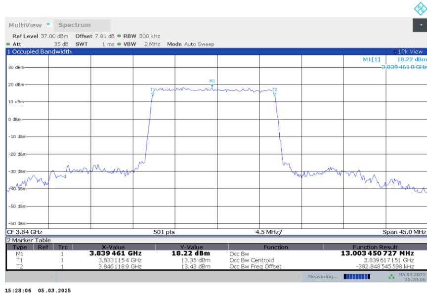
**n77H,15MHz Bandwidth,DFT-s-QPSK (99% BW)**
