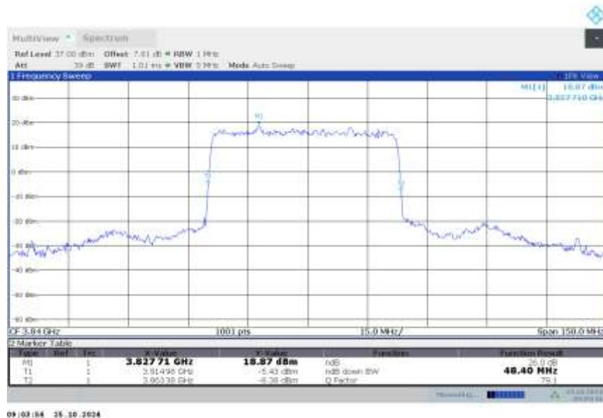
**n77H,50MHz Bandwidth,DFT-s-QPSK (-26dBc BW)**
