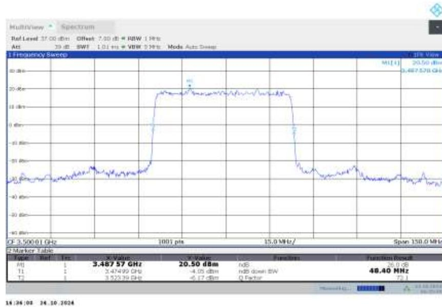
**n77L,50MHz Bandwidth,DFT-s-QPSK (-26dBc BW)**
