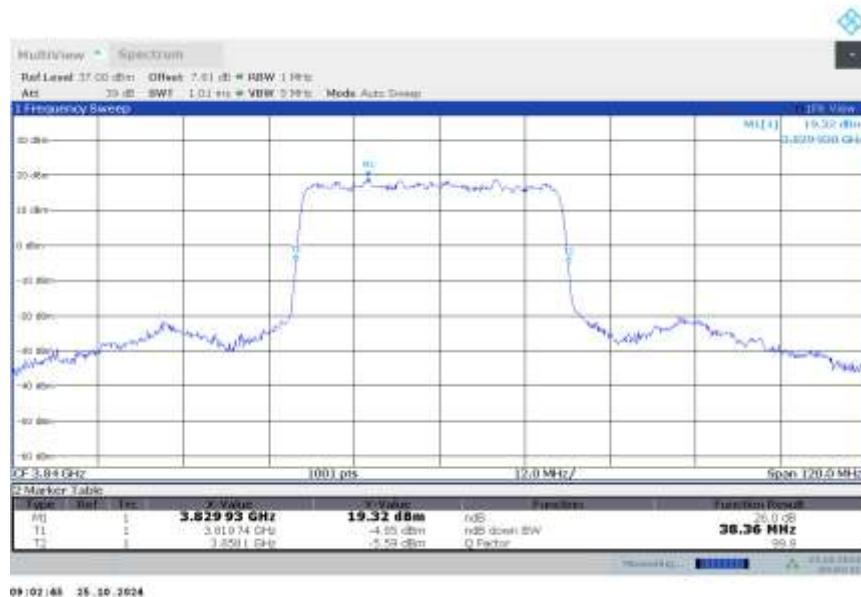
**n77H,40MHz Bandwidth,DFT-s-QPSK (-26dBc BW)**
