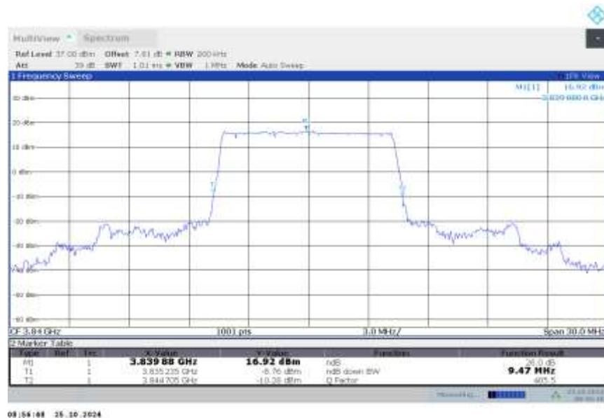
**n77H,10MHz Bandwidth,DFT-s-QPSK (-26dBc BW)**
