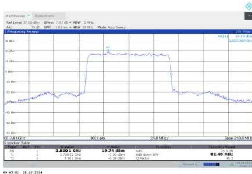
**n77H,80MHz Bandwidth,DFT-s-QPSK (-26dBc BW)**
