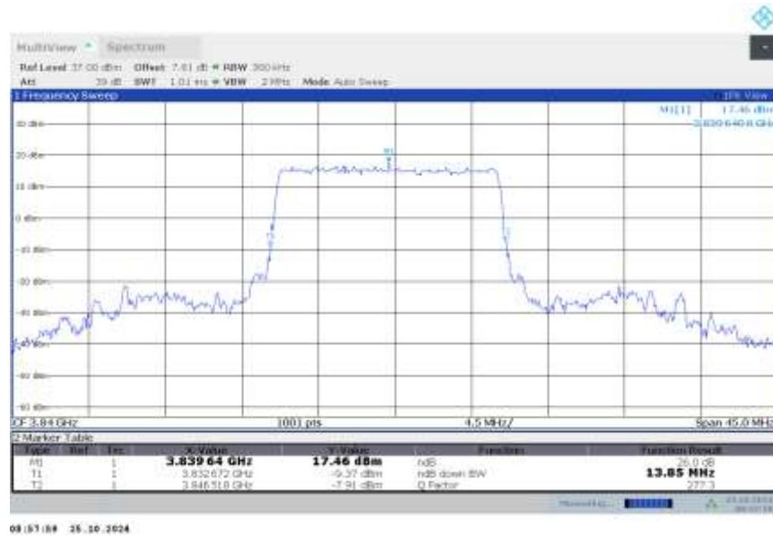
**n77H,15MHz Bandwidth,DFT-s-QPSK (-26dBc BW)**
