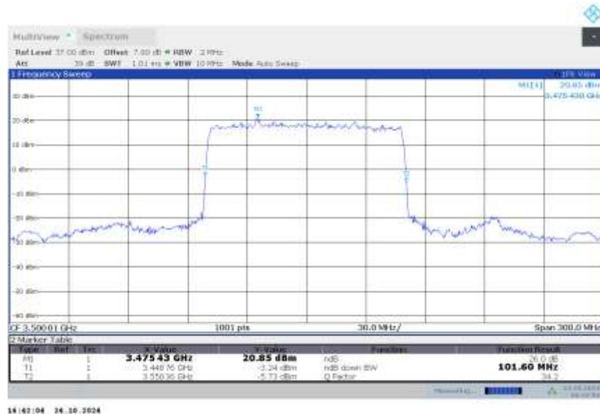
**n77L,100MHz Bandwidth,DFT-s-QPSK (-26dBc BW)**
