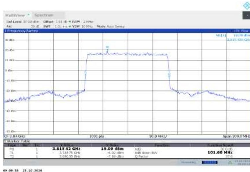
**n77H,100MHz Bandwidth,DFT-s-QPSK (-26dBc BW)**
