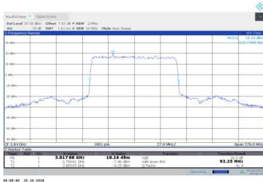
**n77H,90MHz Bandwidth,DFT-s-QPSK (-26dBc BW)**
