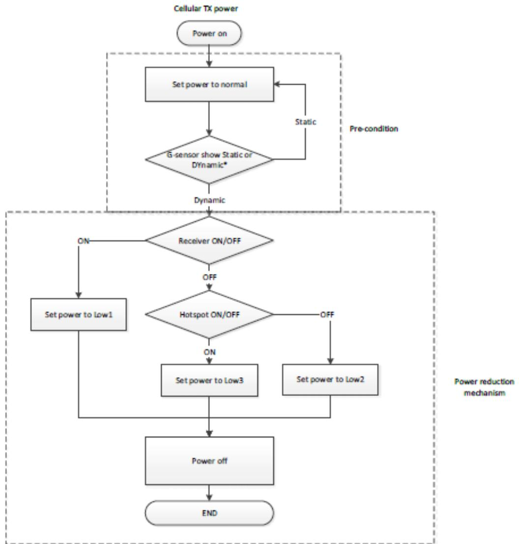
\*When it is in "static" state, the detection frequency is 200ms. When it is In "Dynamic" state, the detection frequency is 30s.
