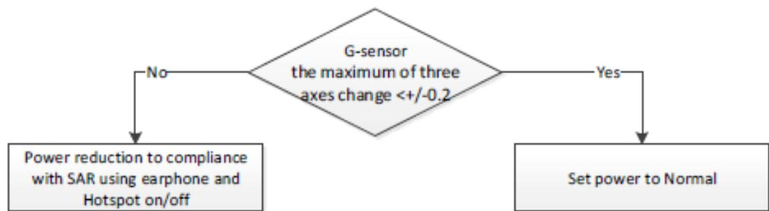
When the maximum of three axes change  $<+/-0.2$ , the user case **MUST be** mobile phone stay away from the body, but if it is  $>+/-0.2$ , it **MAY be** on the person's body, power reduction is on.
