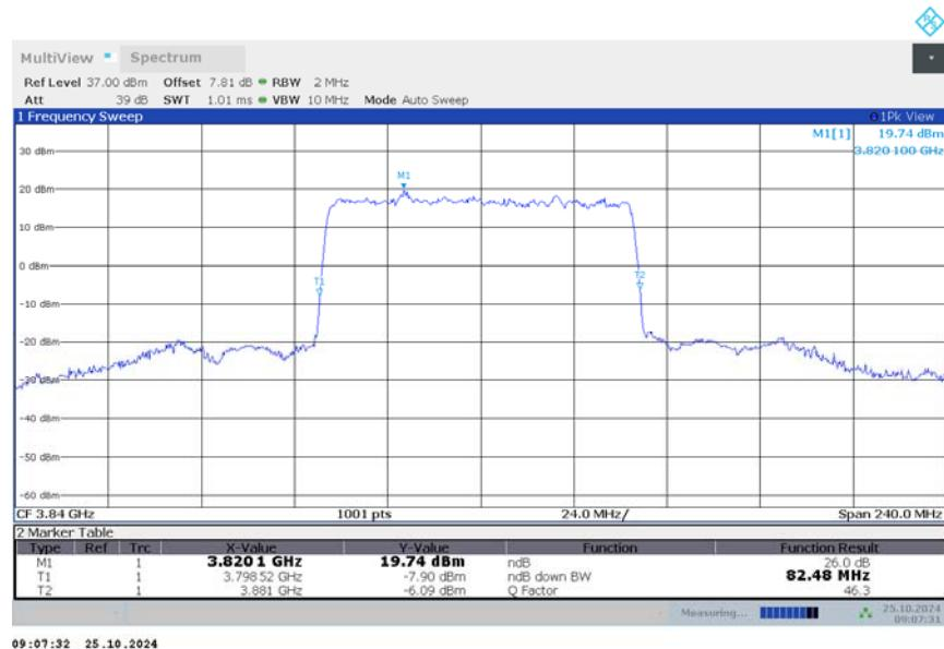
**n77H,80MHz Bandwidth,DFT-s-QPSK (-26dBc BW)**
