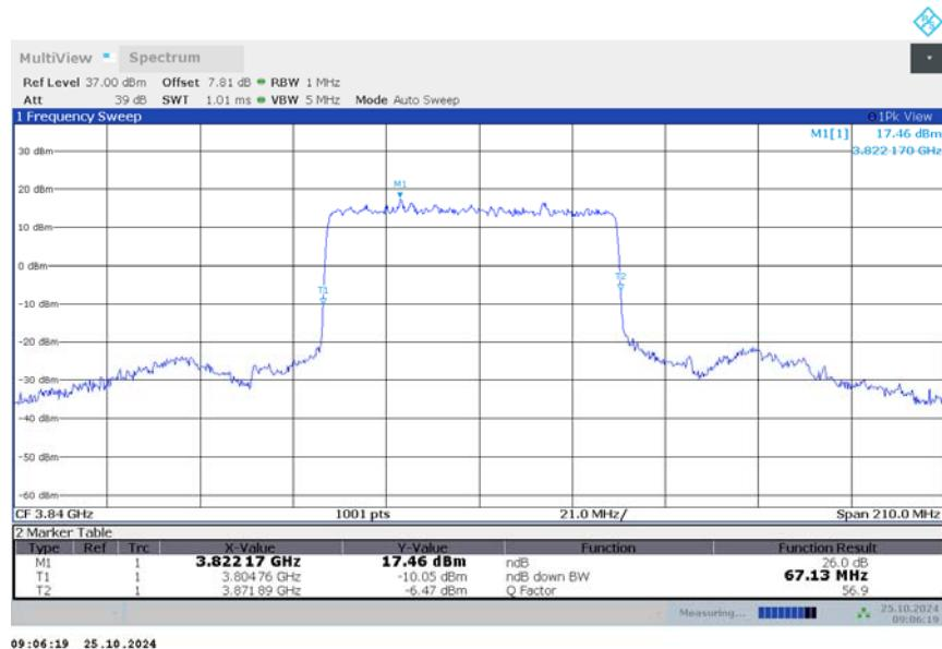
**n77H,70MHz Bandwidth,DFT-s-QPSK (-26dBc BW)**
