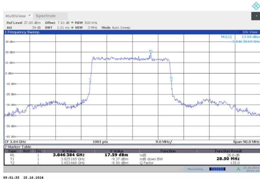
n77H,30MHz Bandwidth,DFT-s-QPSK (-26dBc BW)
