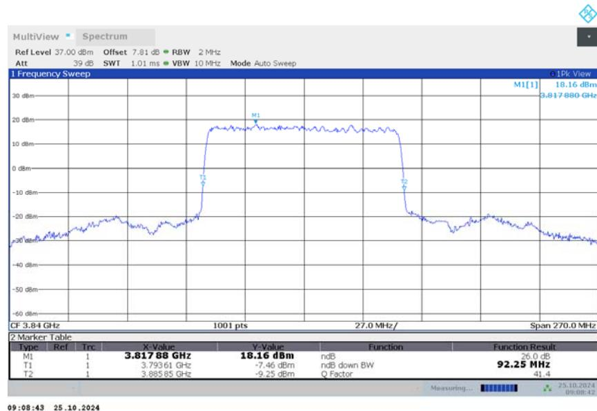
**n77H,90MHz Bandwidth,DFT-s-QPSK (-26dBc BW)**
