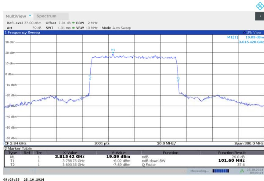
**n77H,100MHz Bandwidth,DFT-s-QPSK (-26dBc BW)**
