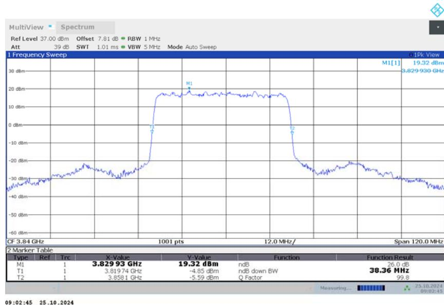
n77H,40MHz Bandwidth,DFT-s-QPSK (-26dBc BW)
