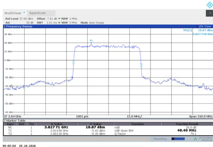
n77H,50MHz Bandwidth,DFT-s-QPSK (-26dBc BW)
