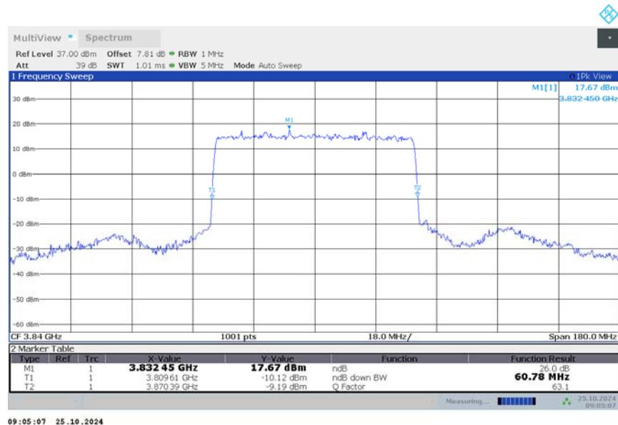
n77H,60MHz Bandwidth,DFT-s-QPSK (-26dBc BW)
