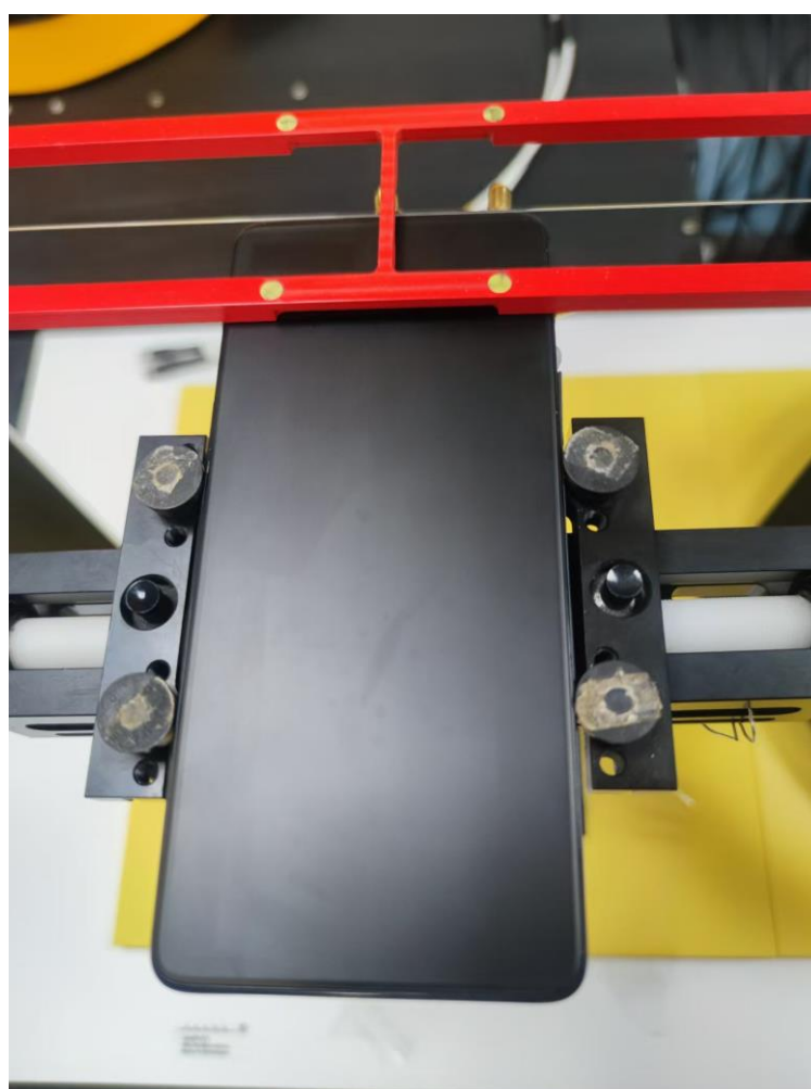
Picture 2: EUT Positioning for RF/T-coil
