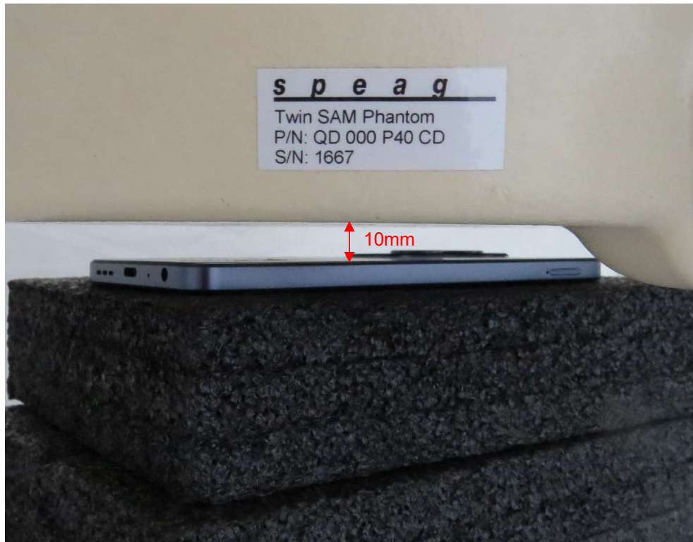
Picture 8: Back Side, the distance from EUT to the bottom of the Phantom is 10mm
