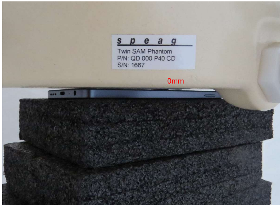
Picture 15: Back Side, the distance from EUT to the bottom of the Phantom is 0mm
