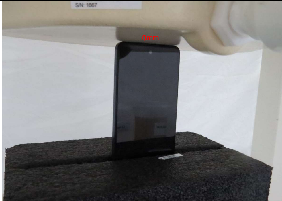
Picture 19: Top Edge, the distance from EUT to the bottom of the Phantom is 0mm
