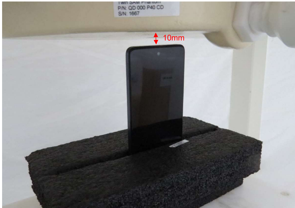
Picture 12: Top Edge, the distance from EUT to the bottom of the Phantom is 10mm
