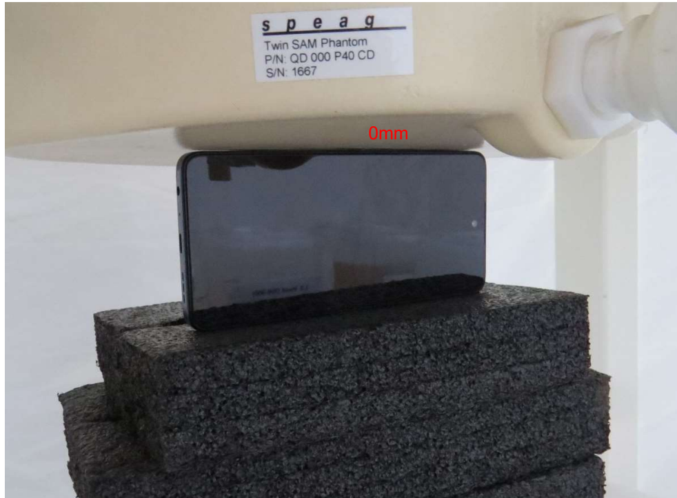
Picture 17: Left Edge, the distance from EUT to the bottom of the Phantom is 0mm
