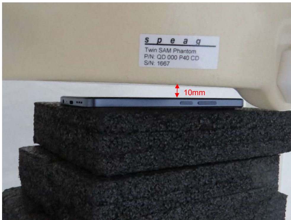
Picture 9: Front Side, the distance from EUT to the bottom of the Phantom is 10mm
