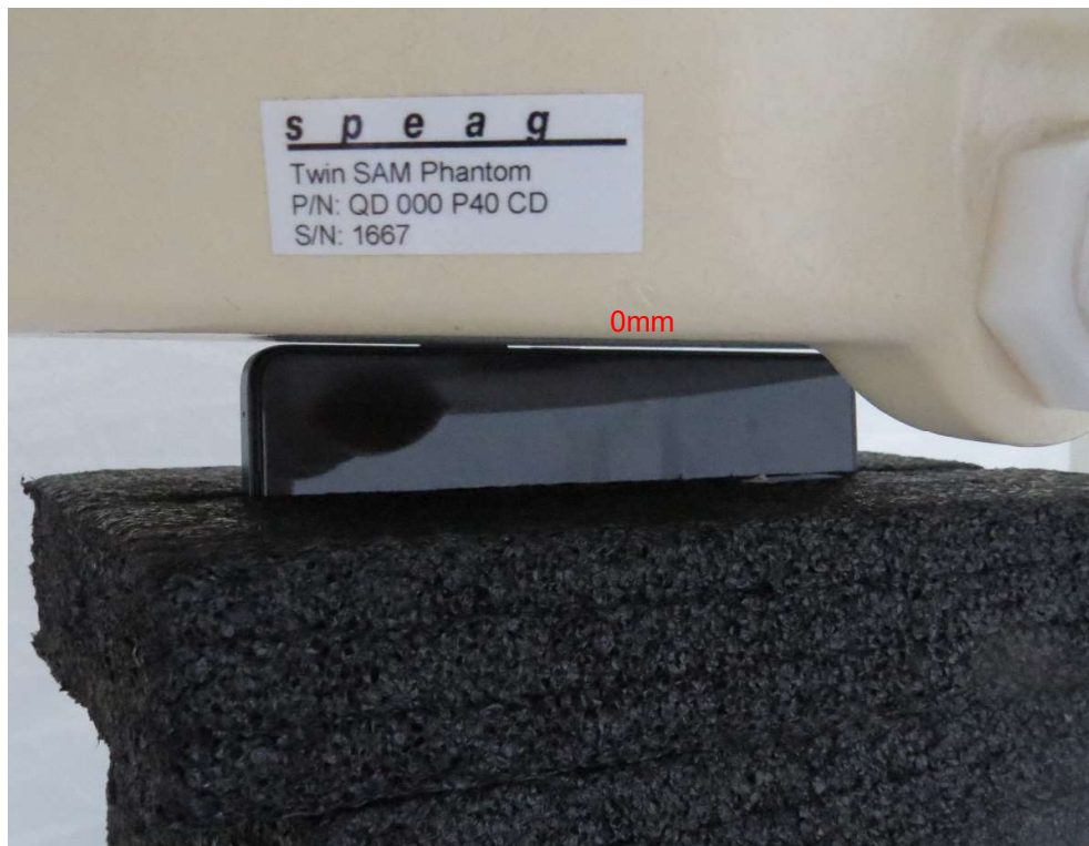
Picture 18: Right Edge, the distance from EUT to the bottom of the Phantom is 0mm
