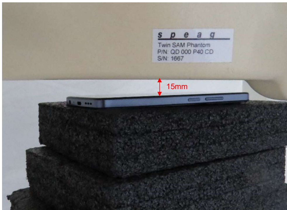
Picture 6: Front Side, the distance from EUT to the bottom of the Phantom is 15mm
