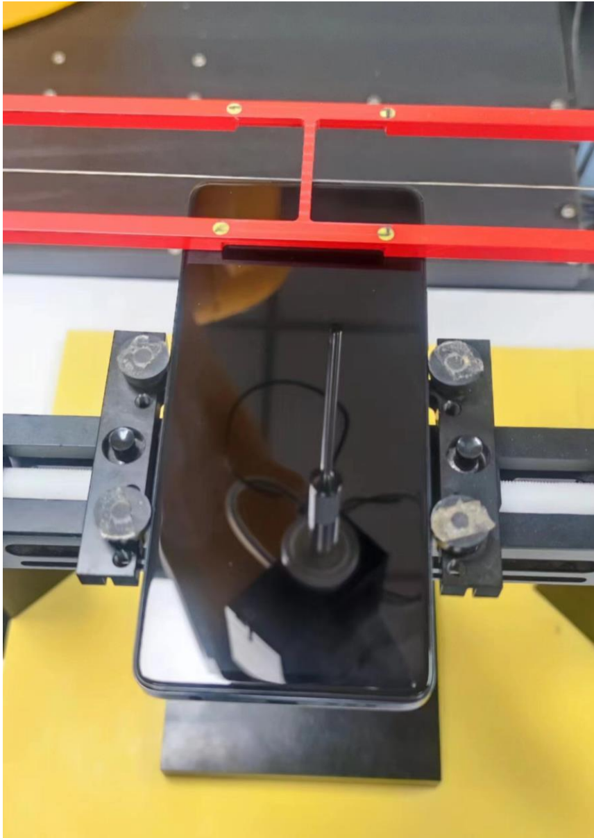
Picture 2: EUT Positioning for RF/T-coil
