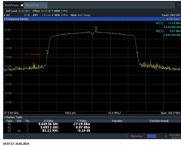
Fig.33 26dB Emission Bandwidth (802. 11ac-VHT80, 5690MHz)
