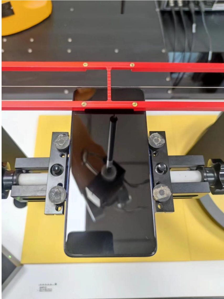
Picture 2: EUT Positioning for RF/T-coil
