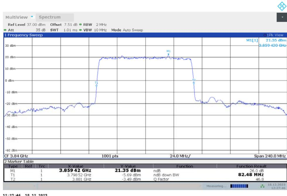
n77H,80MHz Bandwidth,DFT-s-QPSK (-26dBc BW)
