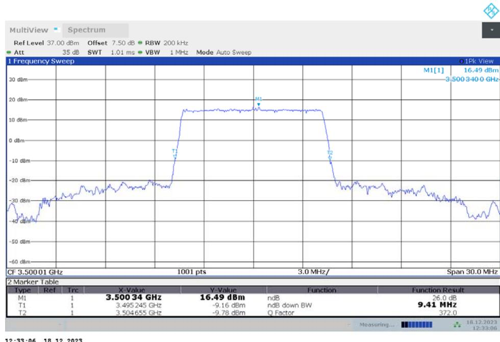
**n78L,10MHz Bandwidth,DFT-s-QPSK (-26dBc BW)**
