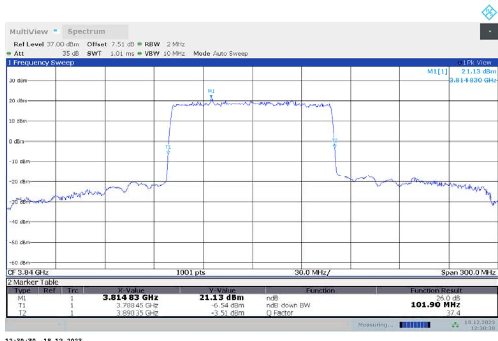
**n77H,100MHz Bandwidth,DFT-s-QPSK (-26dBc BW)**
