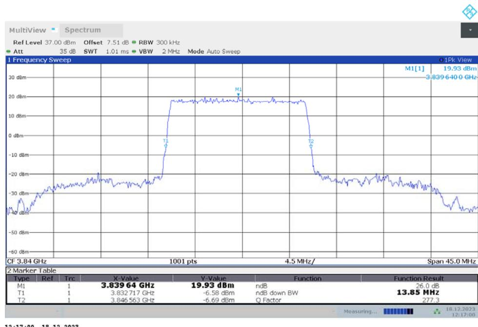
**n77H,15MHz Bandwidth,DFT-s-QPSK (-26dBc BW)**
