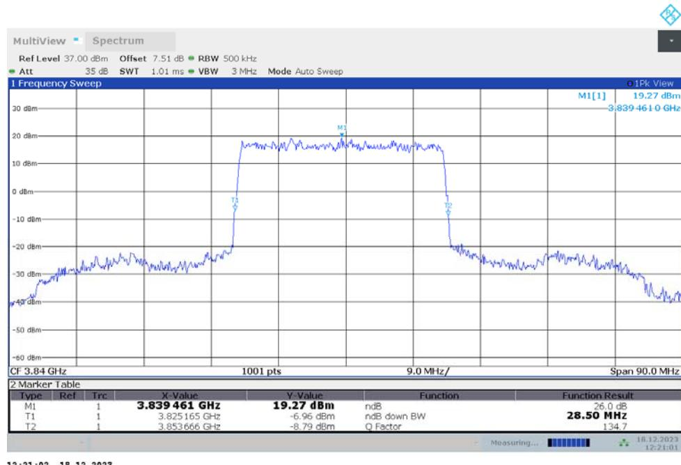
n77H,30MHz Bandwidth,DFT-s-QPSK (-26dBc BW)
