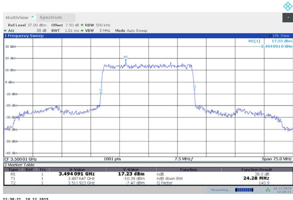
**n78L,25MHz Bandwidth,DFT-s-QPSK (-26dBc BW)**
