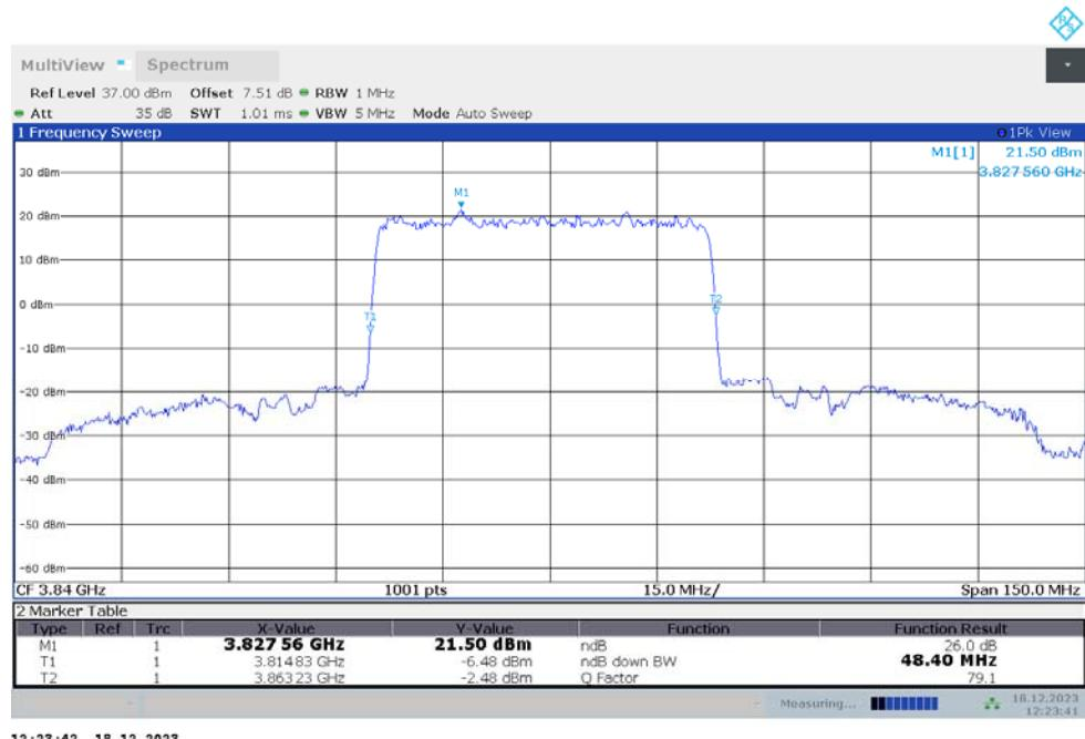
n77H,50MHz Bandwidth,DFT-s-QPSK (-26dBc BW)
