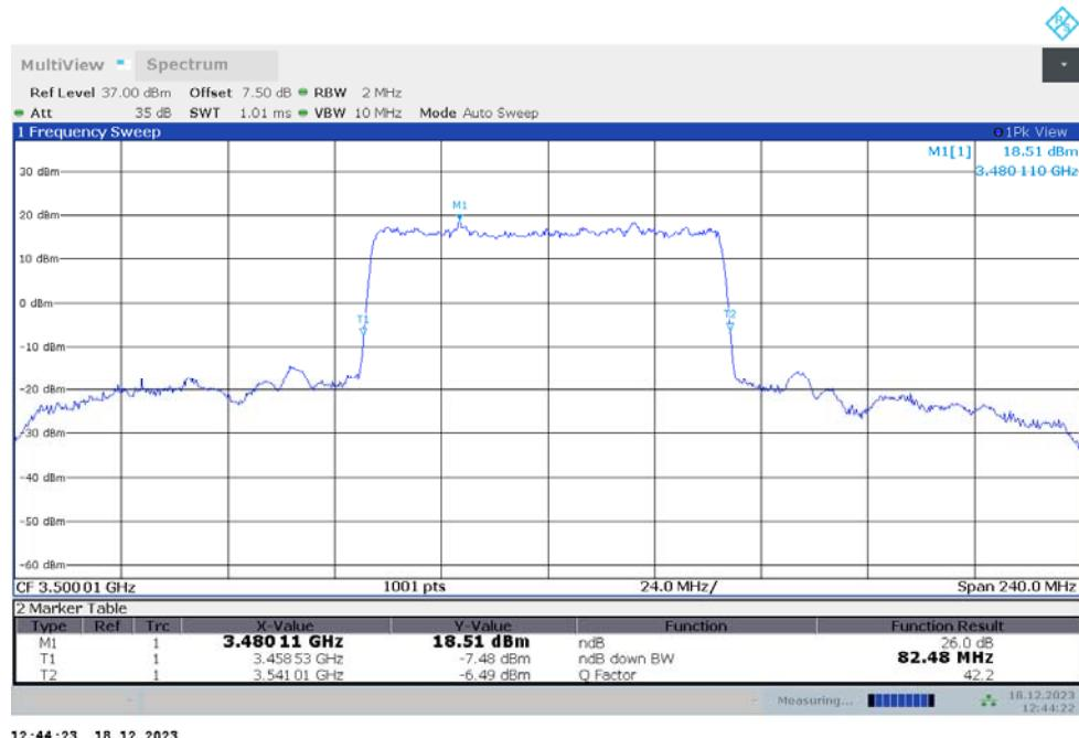
n78L,80MHz Bandwidth,DFT-s-QPSK (-26dBc BW)
