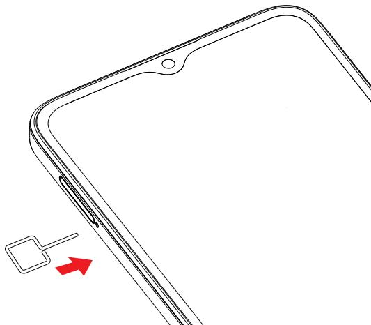
Insert the SIM pin that's provided to eject the SIM tray and then slide it out gently.
