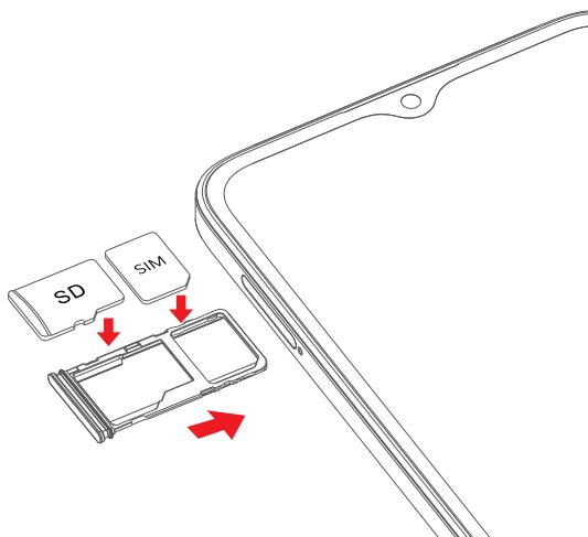
Place or remove the Nano SIM card and the microSD™ card in the correct slot as shown.
