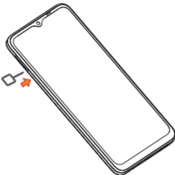
**Step 2.** Remove the NANO SIM card/microSD™ card tray.
