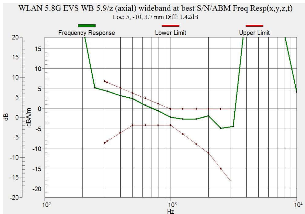
Figure B.23 Frequency Response of WLAN 5.8GHz
