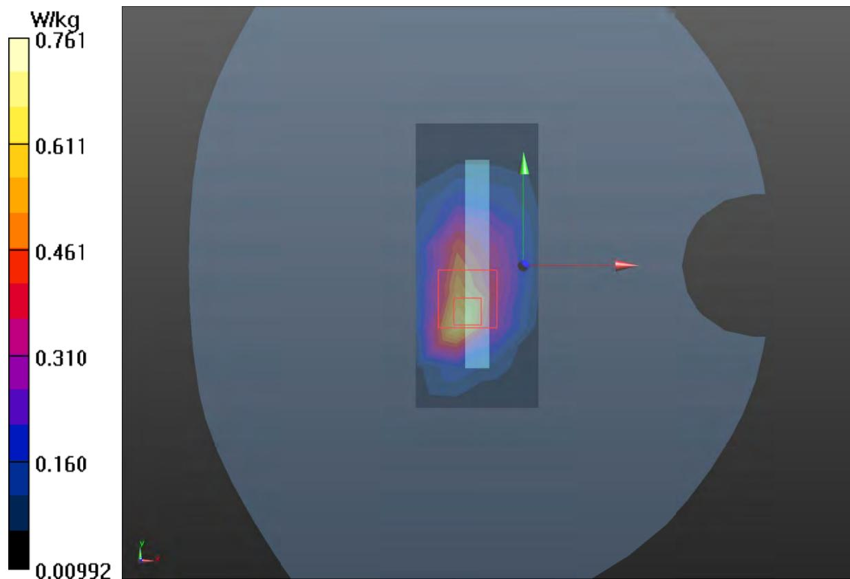
**Plot 71 LTE Band 2 1RB Back Side High (Distance 10mm)**
