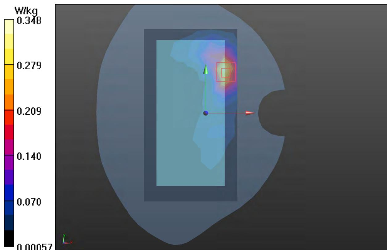
**Plot 57 LTE Band 12 1RB Back Side High (Distance 15mm)**
