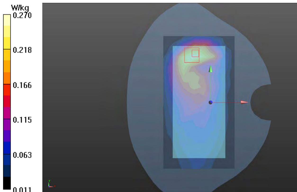
**Plot 59 LTE Band 66 1RB Back Side High (Distance 15mm)**
