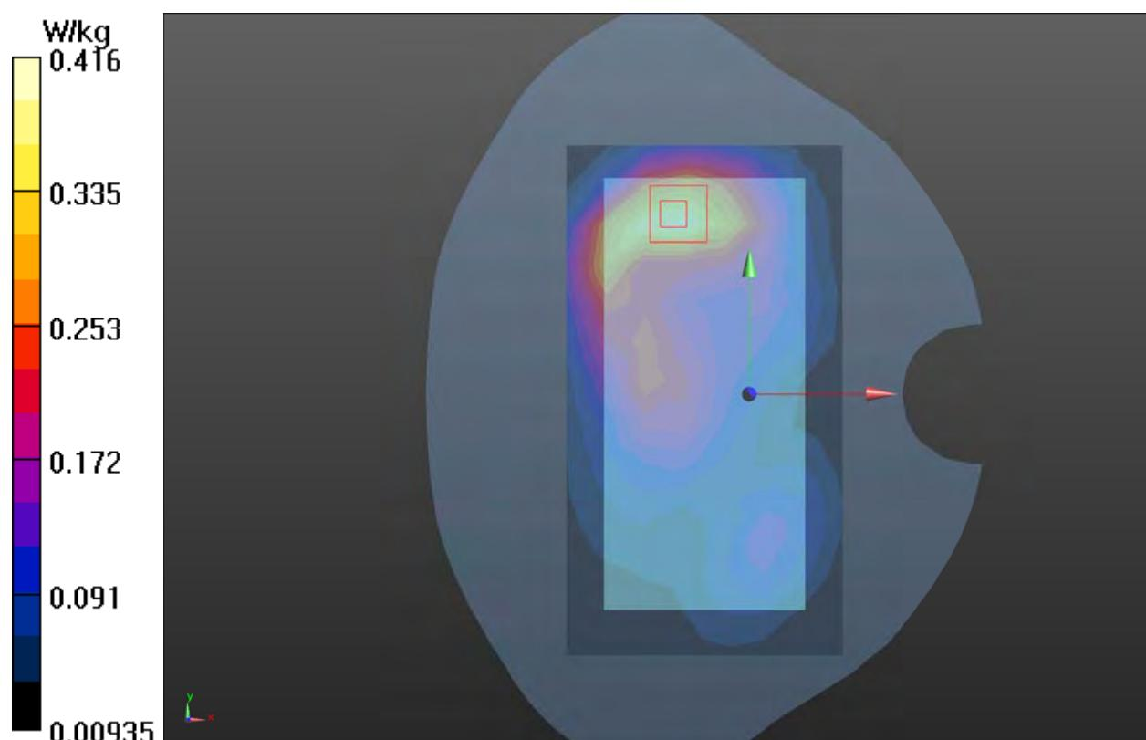
**Plot 54 LTE Band 4 1RB Back Side Low (Distance 15mm)**
