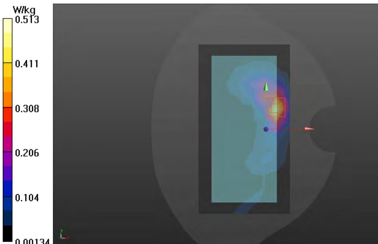
**Plot 72 LTE Band 48 1RB Back Side High (Distance 15mm)**
