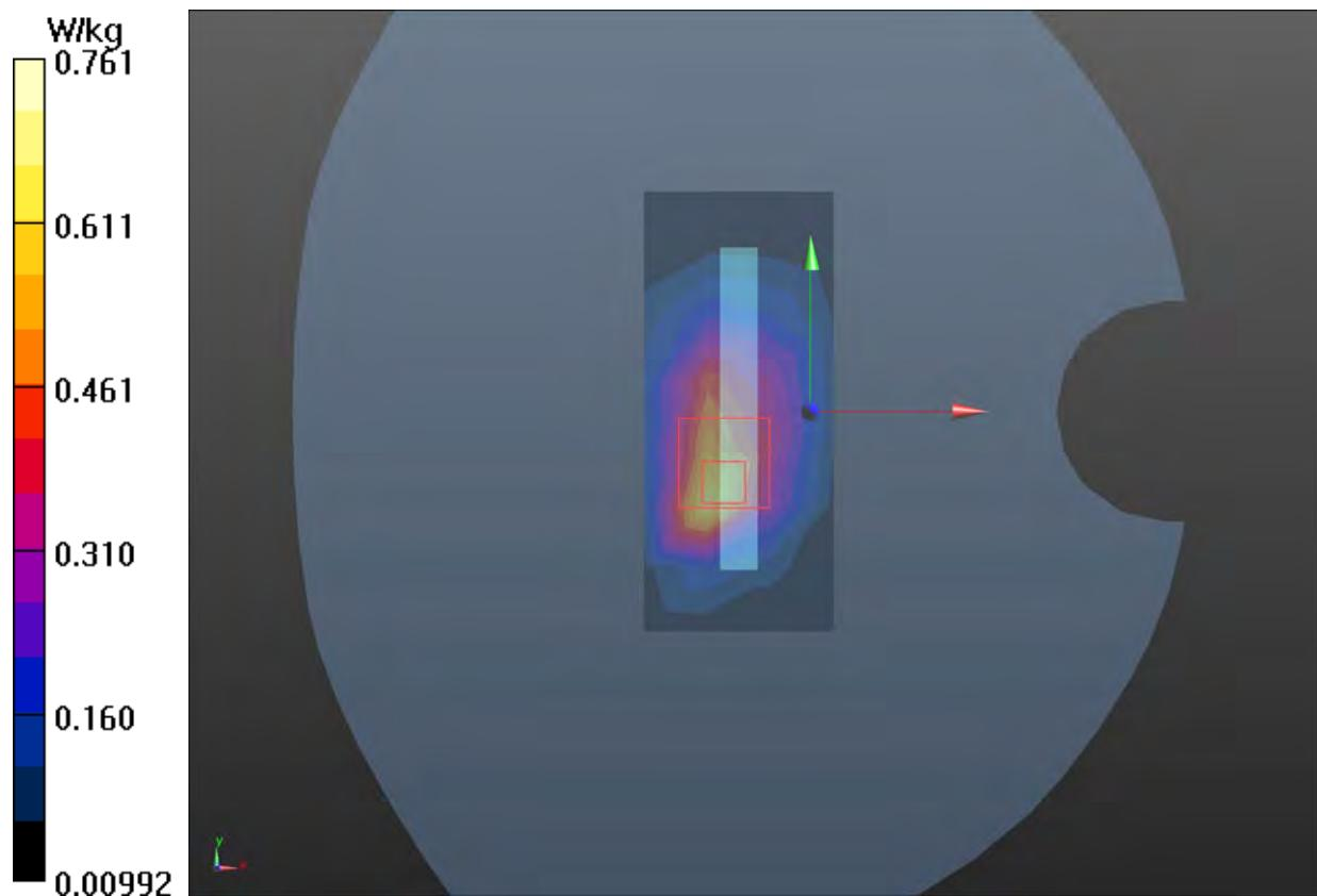
**Plot 90 LTE Band 2 1RB Back Side High (Distance 10mm)**
