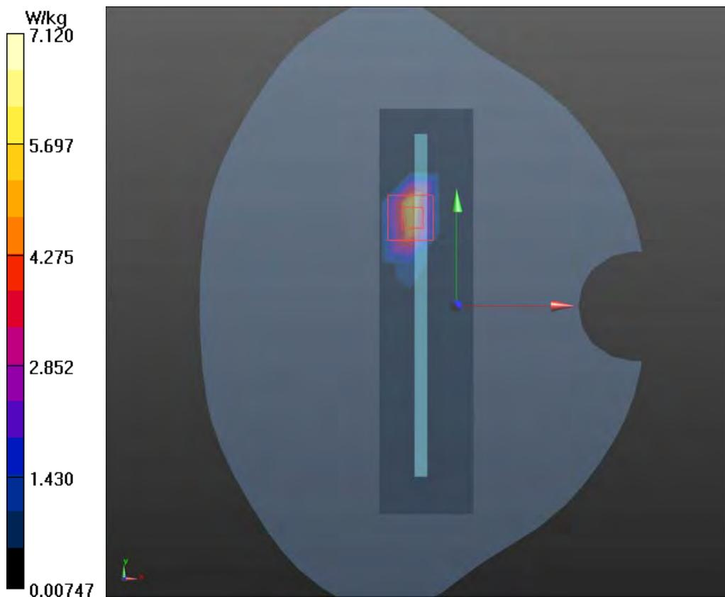
**Plot 115 LTE Band 41 1RB Front Side Middle (Distance 0mm)**
