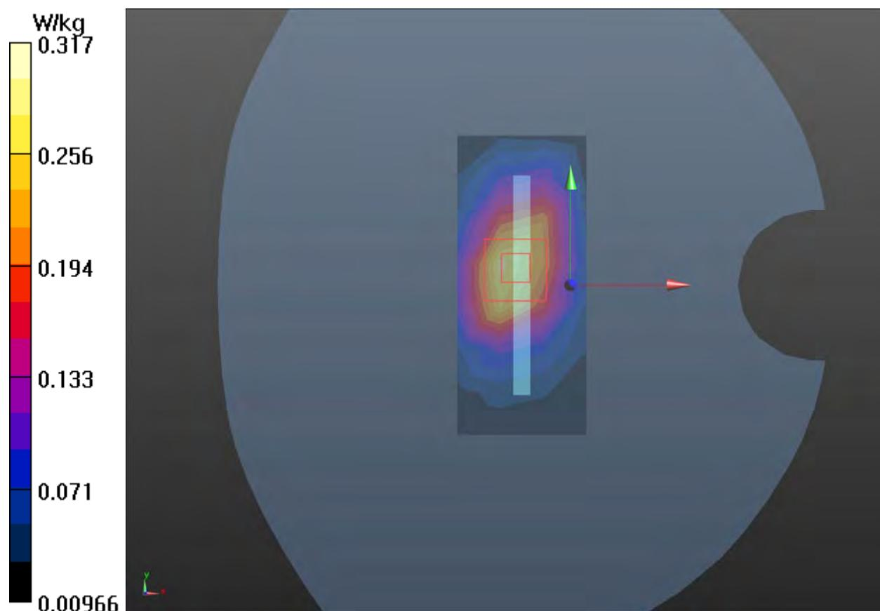
**Plot 101 LTE Band 71 1RB Back Side Low (Distance 10mm)**
