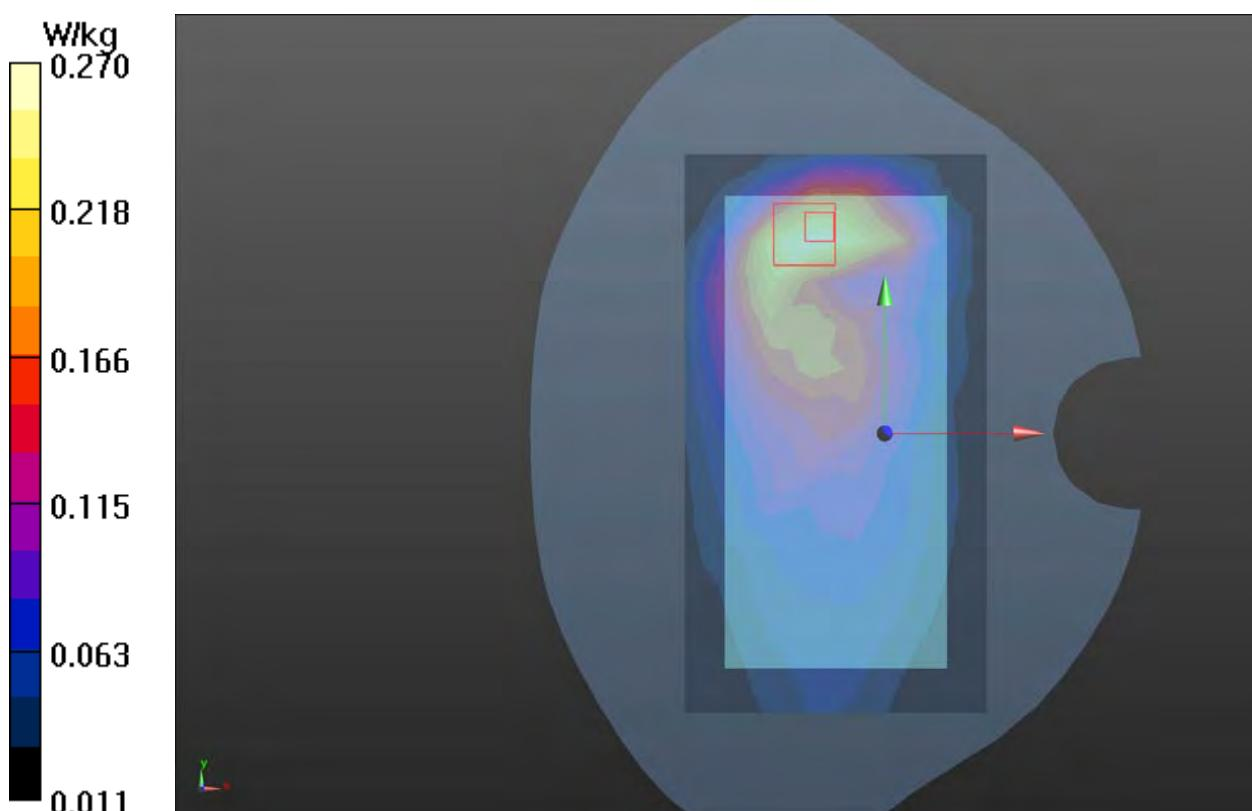
**Plot 69 LTE Band 25 1RB Back Side High (Distance 15mm)**
