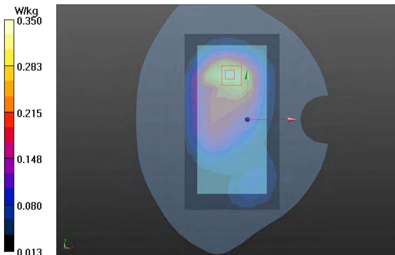
**Plot 74 LTE Band 71 1RB Back Side Low (Distance 15mm)**
