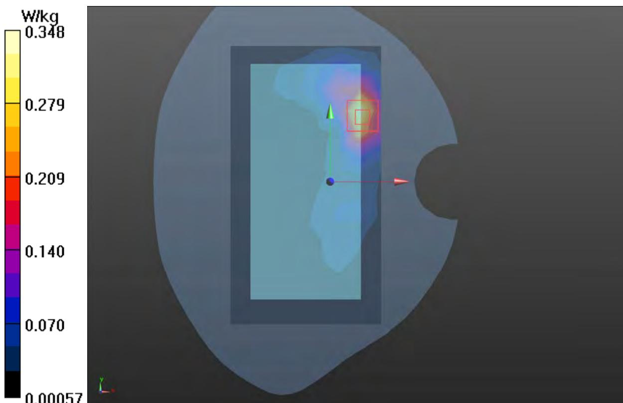
**Plot 67 LTE Band 12 1RB Back Side High (Distance 15mm)**
