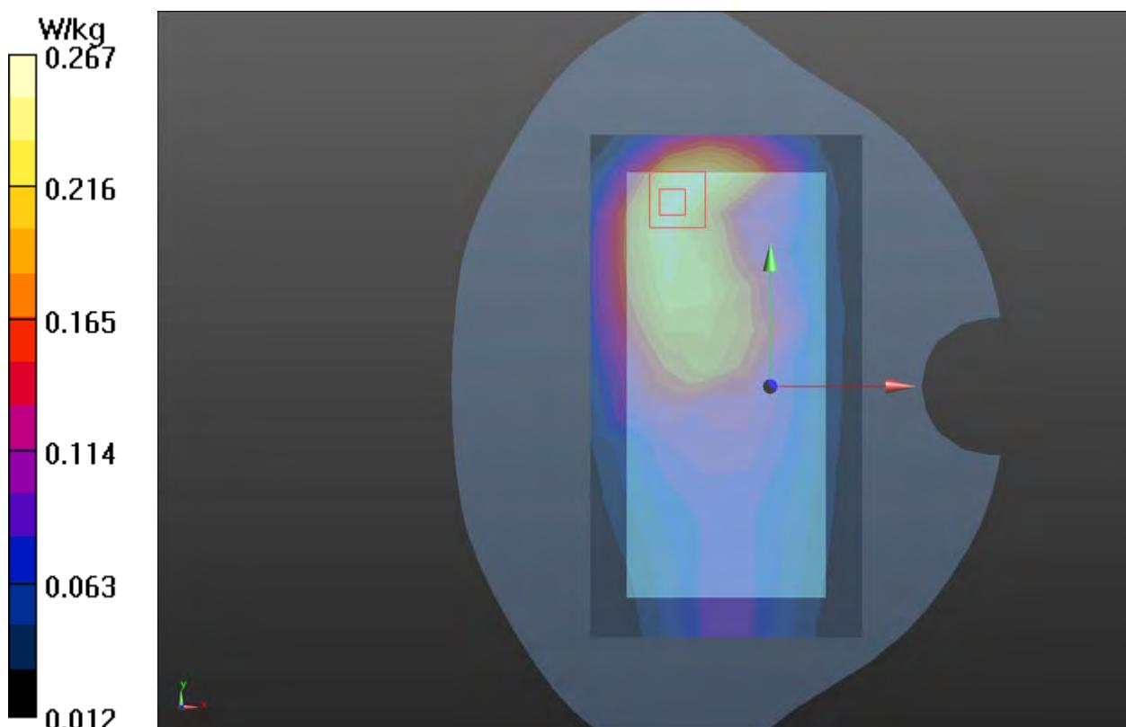
**Plot 71 LTE Band 41 1RB Back Side High (Distance 15mm)**
