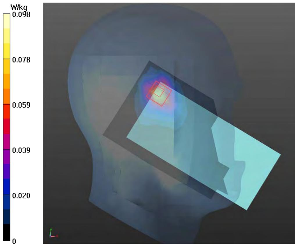
**Plot 58 GSM 850 Back Side Middle (Distance 15mm)**
