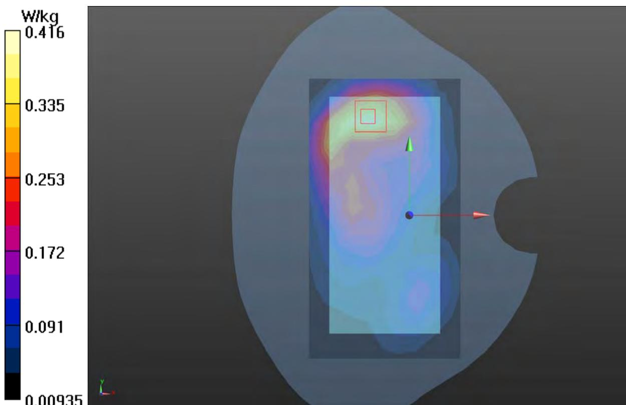
**Plot 64 LTE Band 4 1RB Back Side Low (Distance 15mm)**
