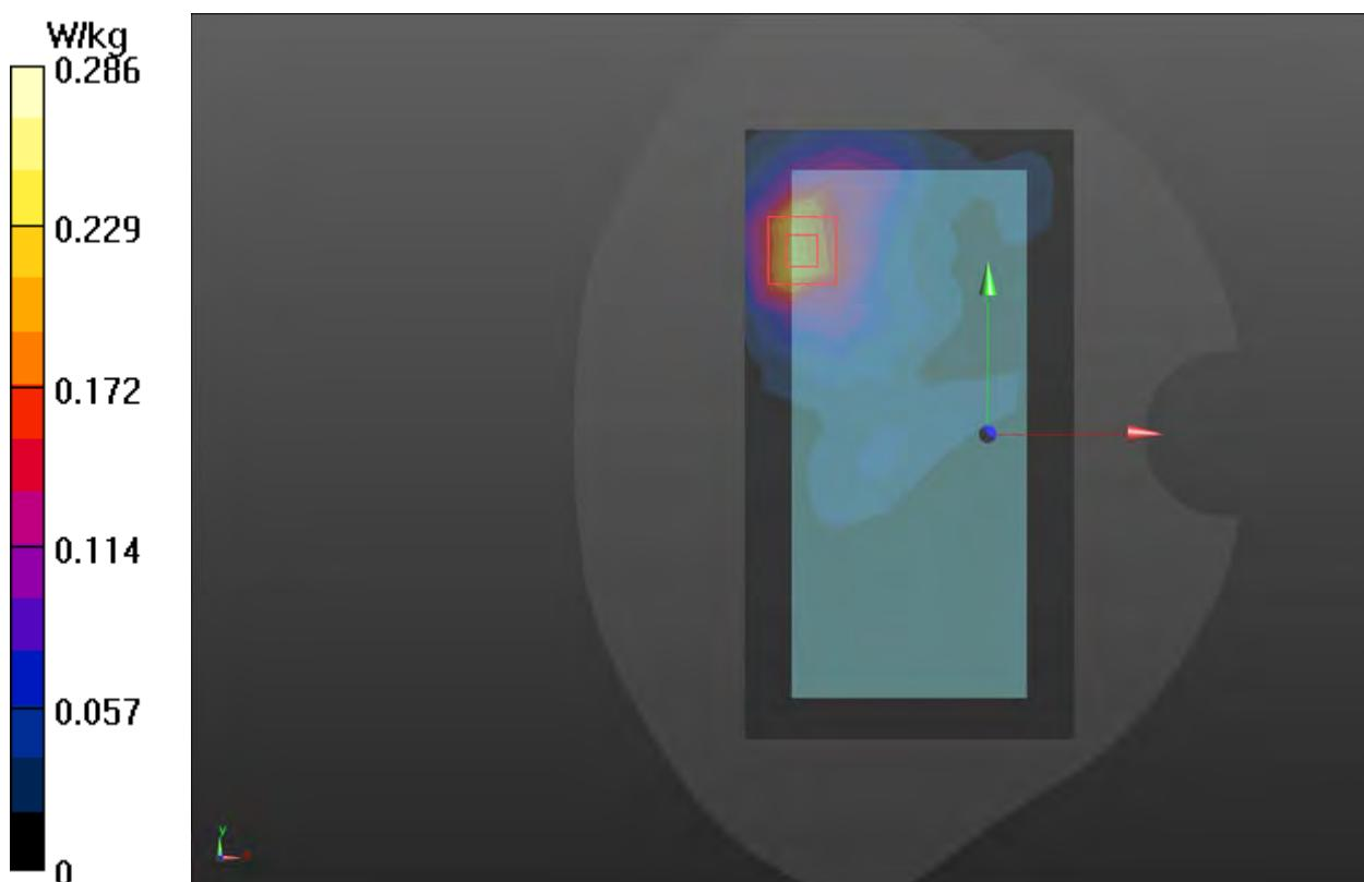
**Plot 73 LTE Band 66 1RB Back Side High (Distance 15mm)**
