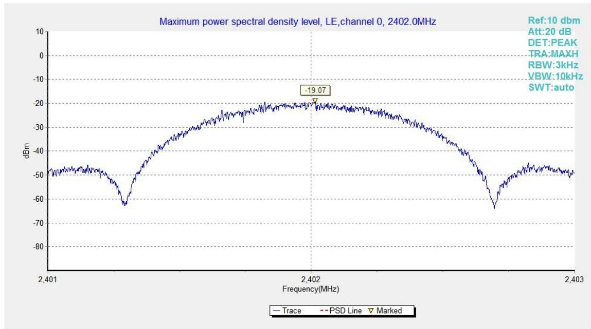
Fig.21. Maximum Power Spectral Density Level Function: GFSK, 2402 MHz
