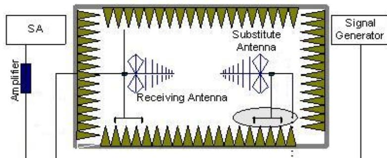
In the chamber, a substitution antenna for the frequency band of interest is placed at the reference point of the chamber. An RF Signal source for the frequency band of interest is connected to the substitution antenna with a cable that has been constructed to not interfere with the radiation pattern of the antenna. A power ( $P_{Mea}$ ) is applied to the input of the substitution antenna, and adjust the level of the signal generator output until the value of the
