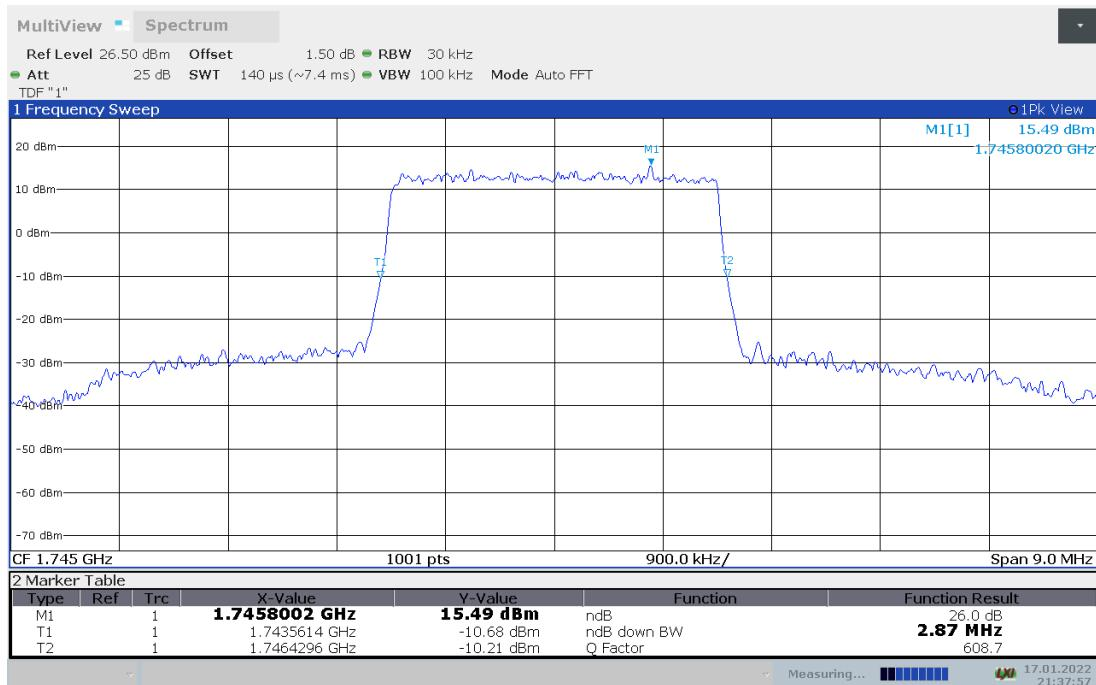
**LTE band 66 , 3MHz Bandwidth,16QAM (-26dBc BW)**
