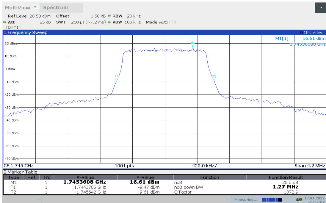
**LTE band 66 , BW1.4MHz Bandwidth,16QAM (-26dBc BW)**
