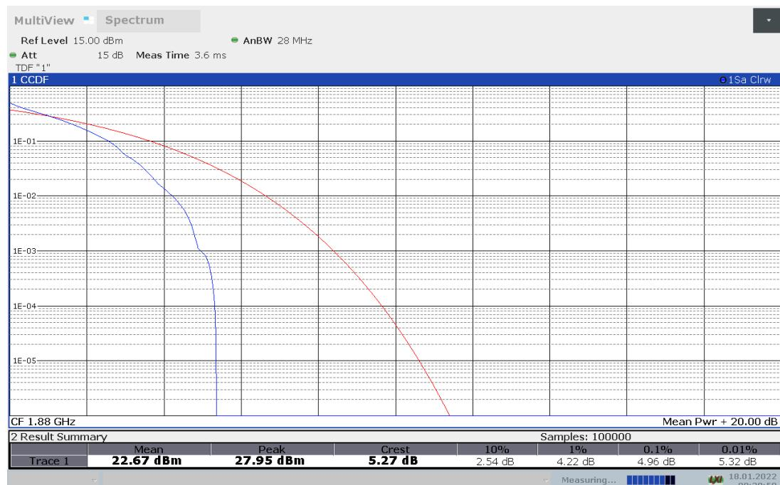
**LTE band 2, 20MHz Bandwidth, 16QAM (PAPR)**
