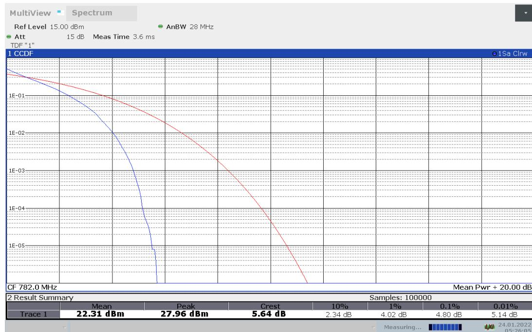
**LTE band 13, 10MHz Bandwidth, 16QAM (PAPR)**
