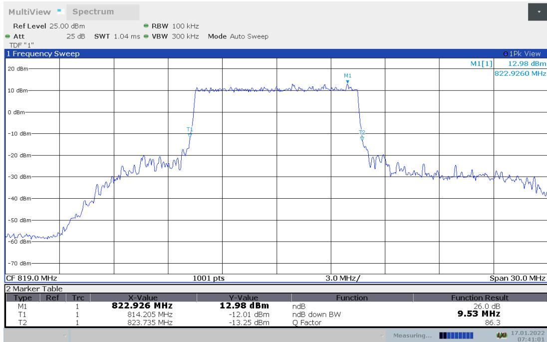
**LTE band 26(814MHz-824MHz), 10MHz Bandwidth,16QAM (-26dBc BW)**
