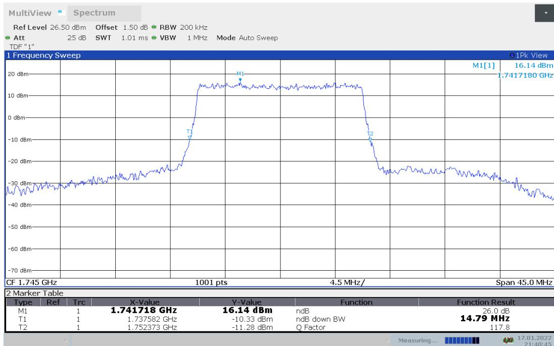
**LTE band 66 , 15MHz Bandwidth,16QAM (-26dBc BW)**
