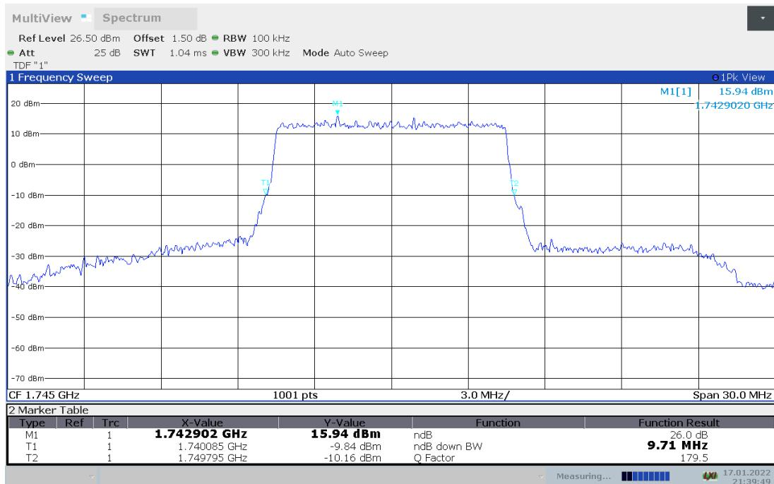
**LTE band 66 , 10MHz Bandwidth,16QAM (-26dBc BW)**
