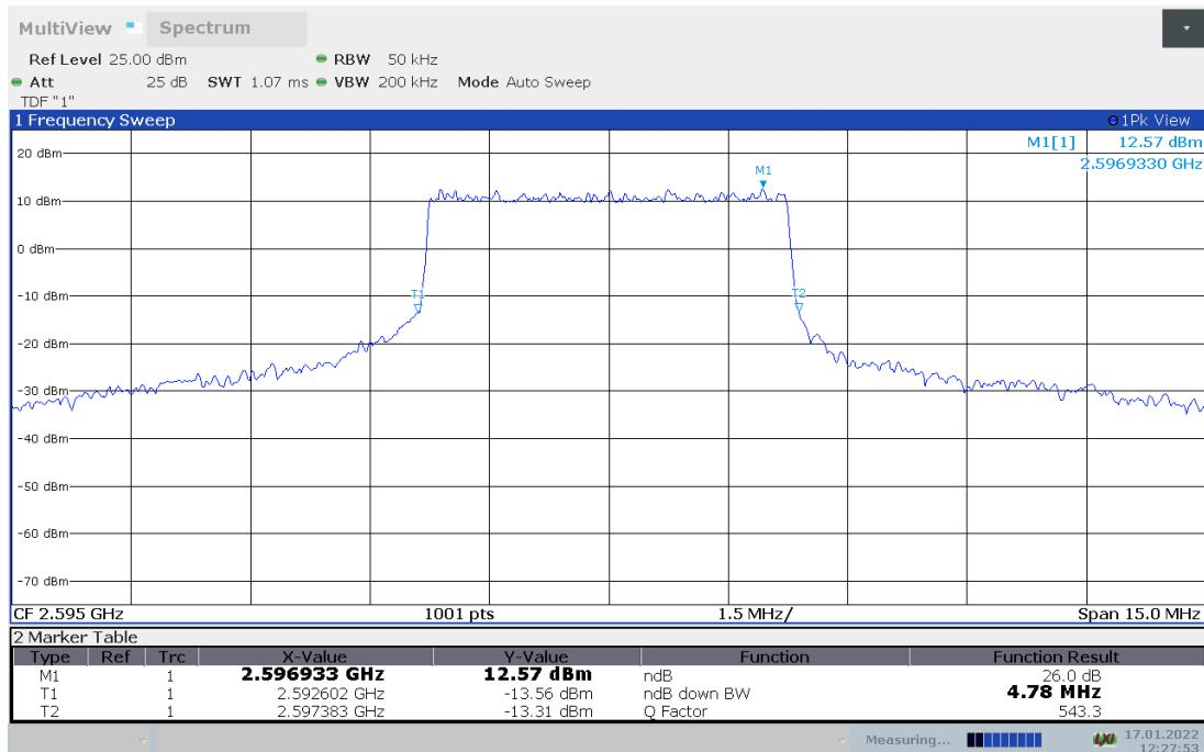
**LTE band 38 , 5MHz Bandwidth,16QAM (-26dBc BW)**
