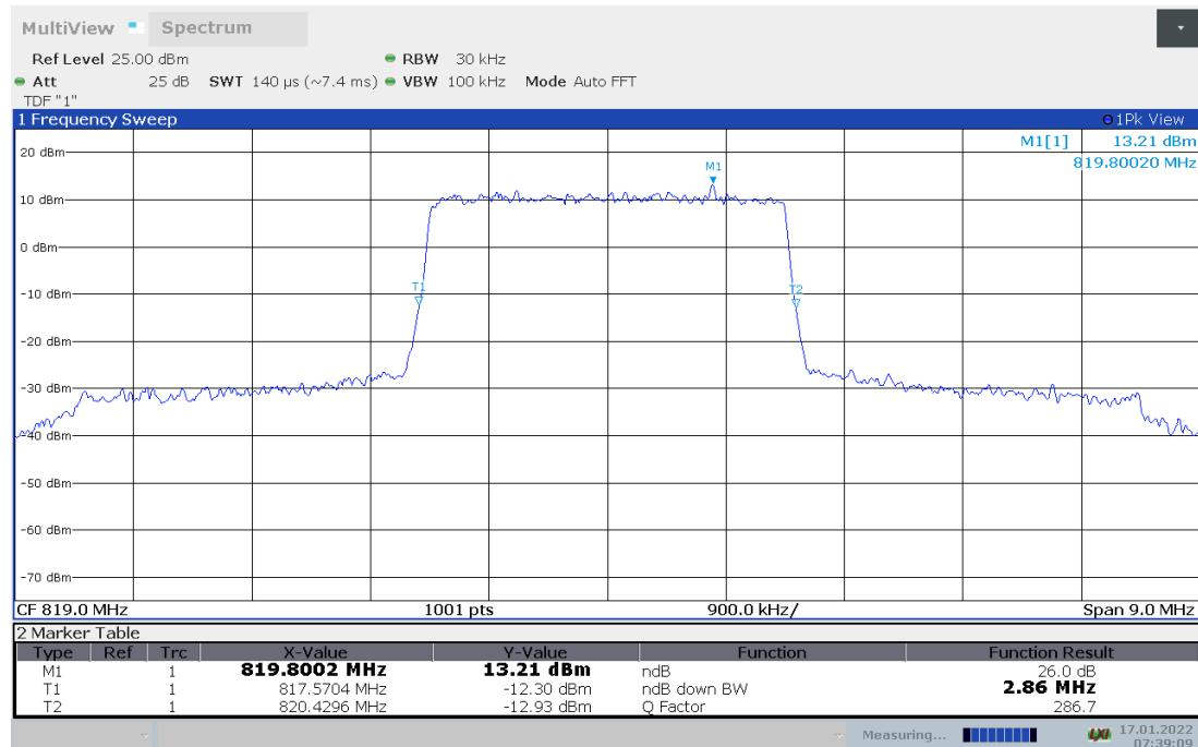
**LTE band 26(814MHz-824MHz), 3MHz Bandwidth,16QAM (-26dBc BW)**
