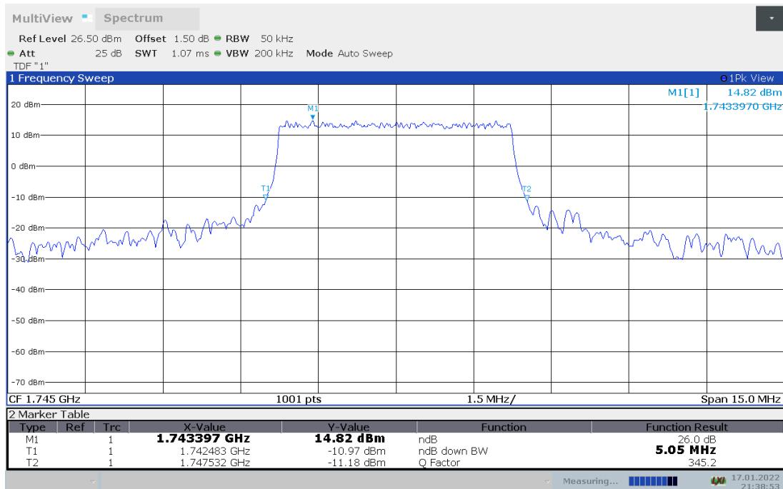
**LTE band 66 , 5MHz Bandwidth,16QAM (-26dBc BW)**
