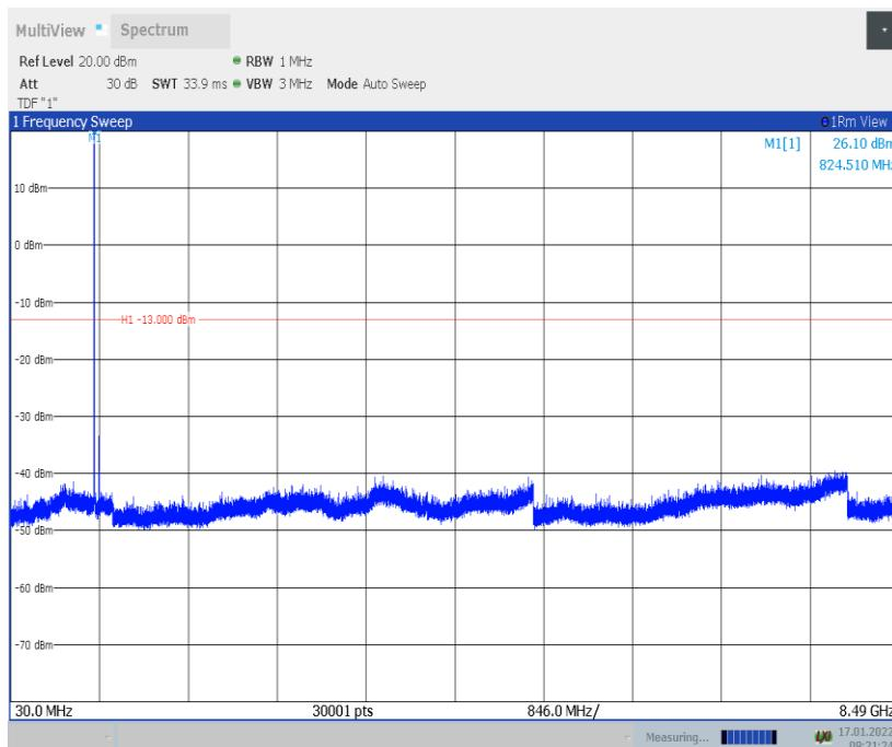
**LTE band 26(824MHz-849MHz): 30MHz – 8.49GHz**
