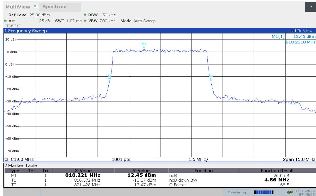
**LTE band 26(814MHz-824MHz), 5MHz Bandwidth,16QAM (-26dBc BW)**
