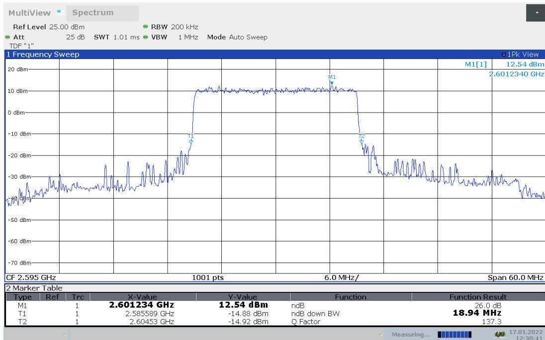
**LTE band 38 , 20MHz Bandwidth,16QAM (-26dBc BW)**
