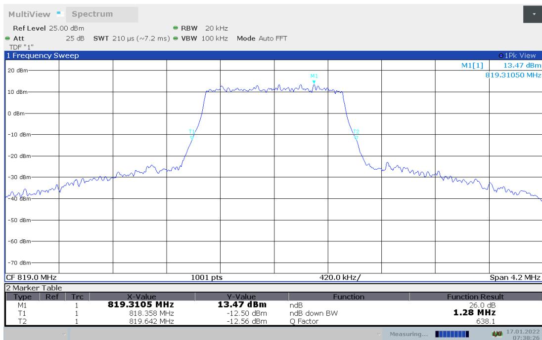
**LTE band 26(814MHz-824MHz),3MHz(-26dBc)**
