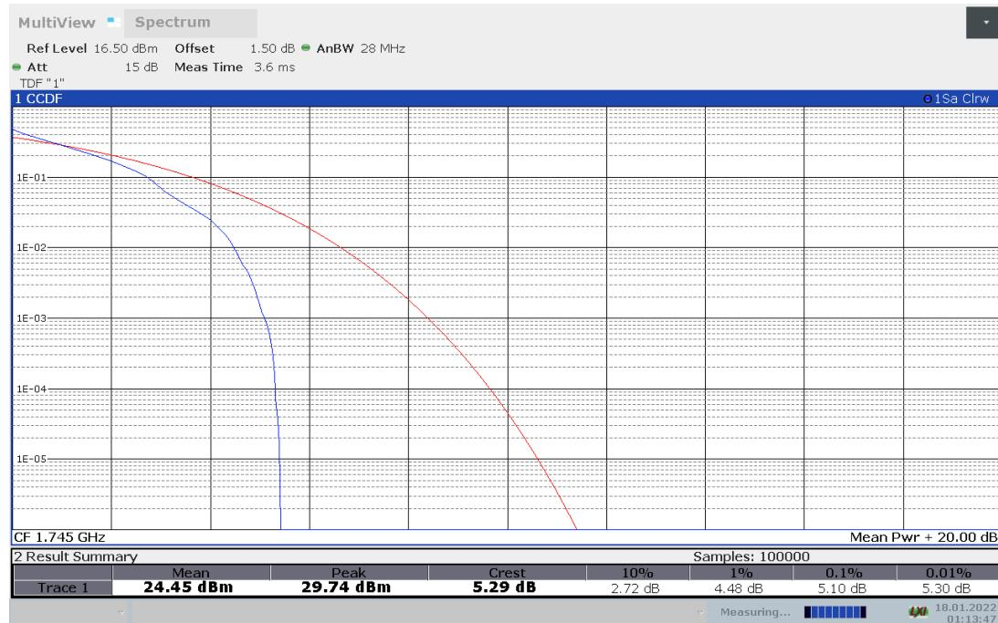
**LTE band 66, 20MHz Bandwidth, 16QAM (PAPR)**
