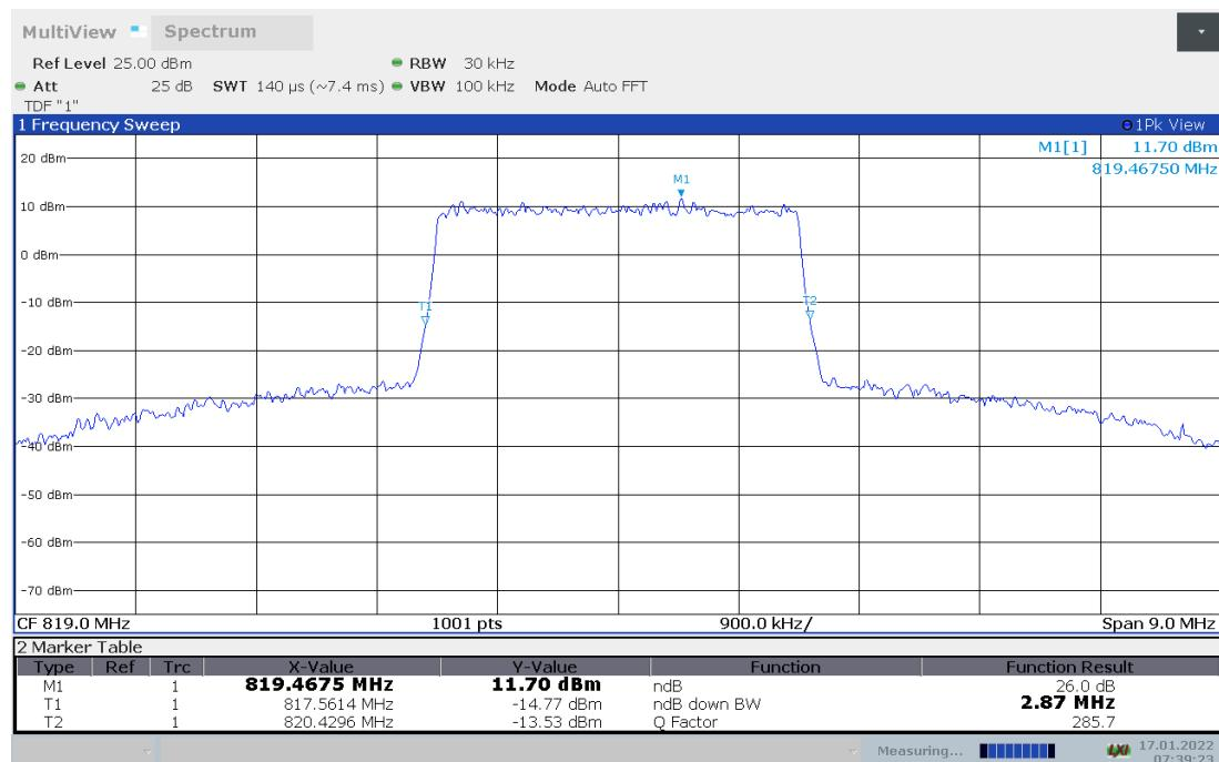
**LTE band 26(814MHz-824MHz),5MHz(-26dBc)**
