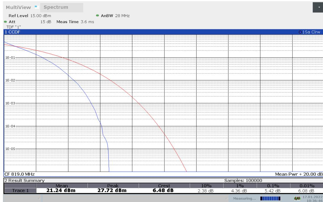
**LTE band 26(814MHz -824MHz), 15MHz Bandwidth, 16QAM (PAPR)**
