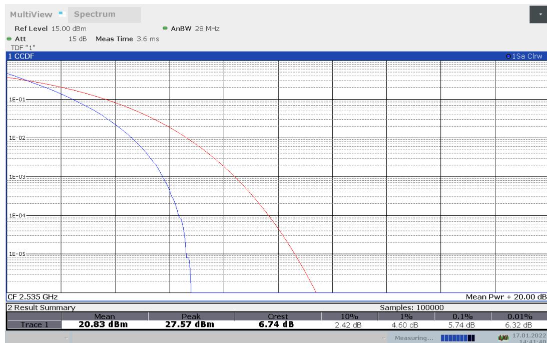
**LTE band 7, 20MHz Bandwidth, 16QAM (PAPR)**
