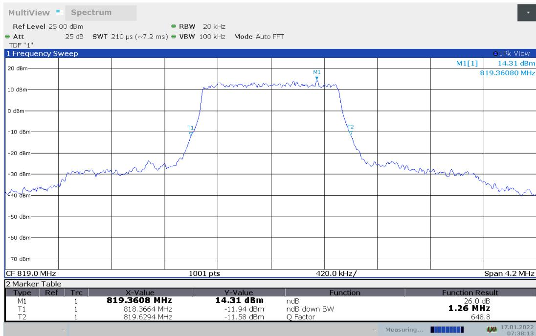
**LTE band 26(814MHz-824MHz), BW1.4MHz Bandwidth,16QAM (-26dBc BW)**
