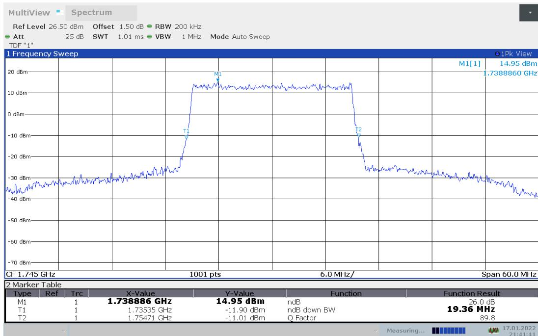
**LTE band 66 , 20MHz Bandwidth,16QAM (-26dBc BW)**
