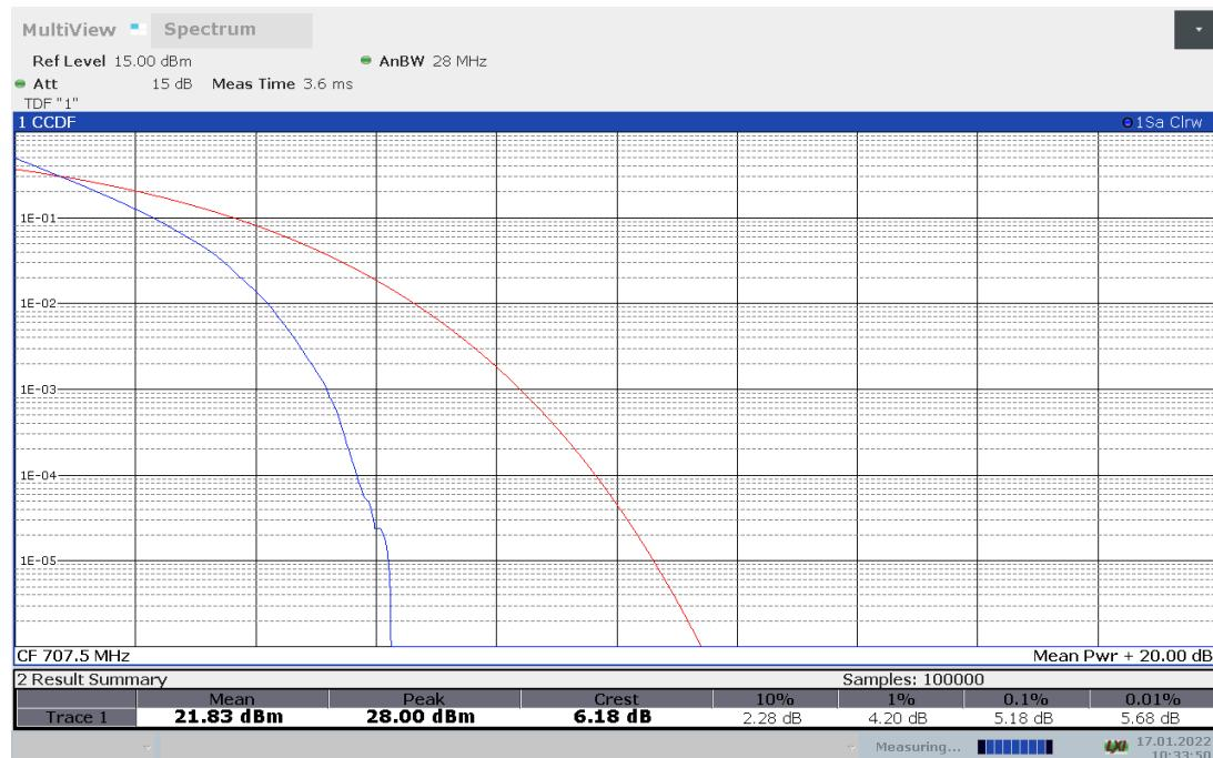
**LTE band 12, 10MHz Bandwidth, 16QAM (PAPR)**
