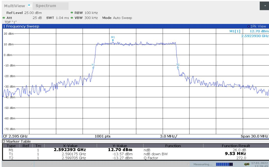
**LTE band 38 , 10MHz Bandwidth,16QAM (-26dBc BW)**
