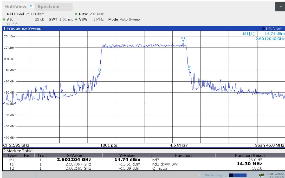
**LTE band 38 , 15MHz Bandwidth,16QAM (-26dBc BW)**
