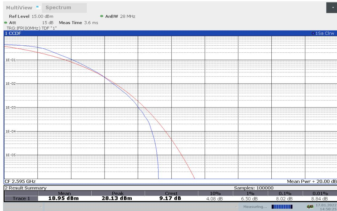
**LTE band 38, 20MHz Bandwidth, 16QAM (PAPR)**
