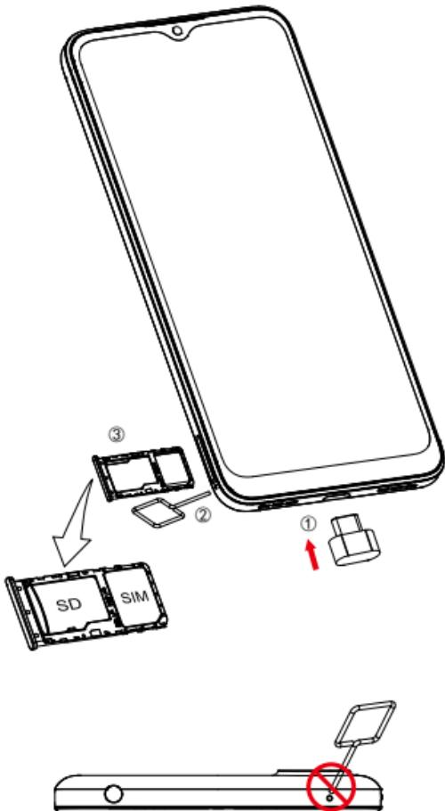
**Caution:** Do not insert the SIM pin into the speaker on top or bottom of the phone.
