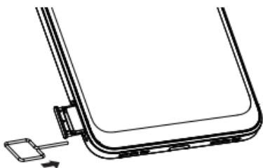
Insert the SIM pin that's provided to eject the SIM tray and then slide it out gently.
