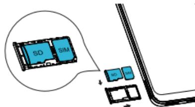
Place or remove the Nano SIM card and the microSD<sup>TM</sup> card in the correct slot as shown.
