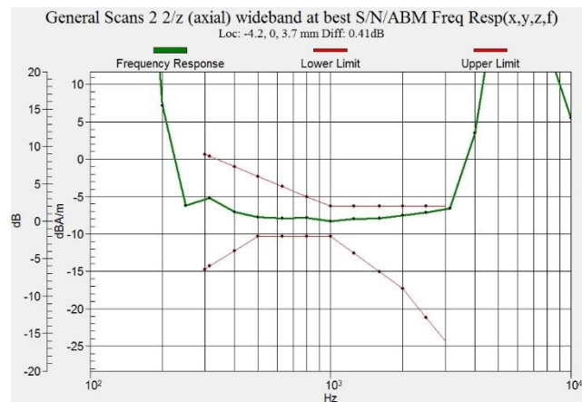
Figure C.5 Frequency Response of WiFi-2.4G
