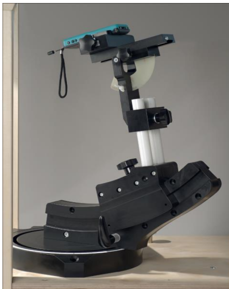
F-2. Device Holder for Transmitters
