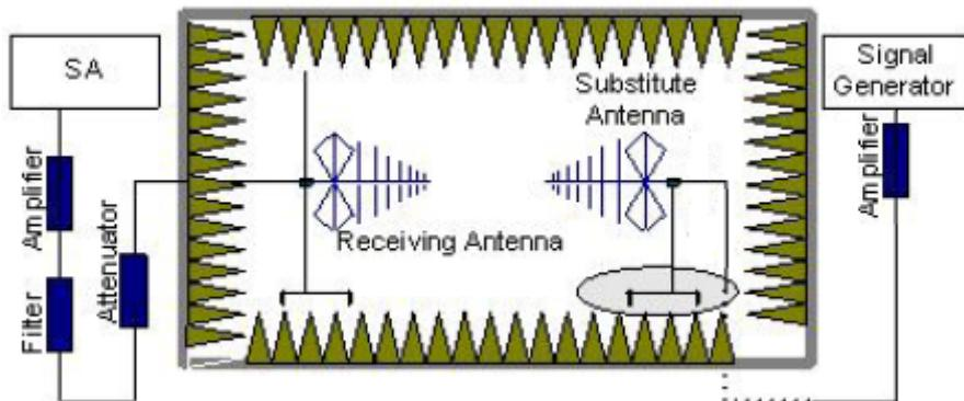
In the chamber, a substitution antenna for the frequency band of interest is placed at the reference point of the chamber. An RF Signal source for the frequency band of interest is connected to the substitution antenna with a cable that has been constructed to not interfere
