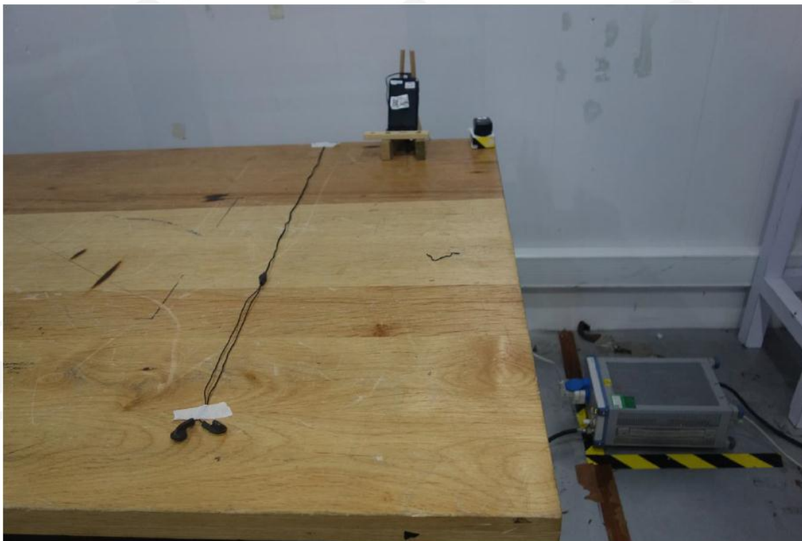
Power Line Conducted Emissions
