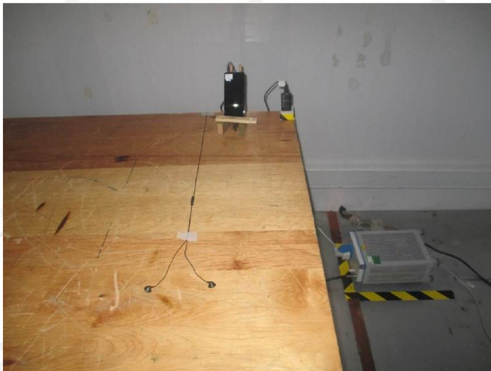
Power Line Conducted Emissions
