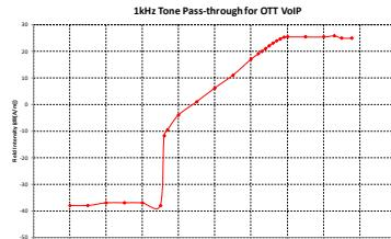
This model was verified to be within the linear region for ABM1 measurements at -20 dBm0 for OTT VoIP. This measurement was taken in the axial configuration above the maximum location.
