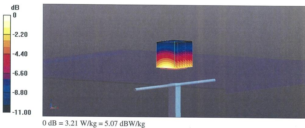
Impedance Measurement Plot for Head TSL
