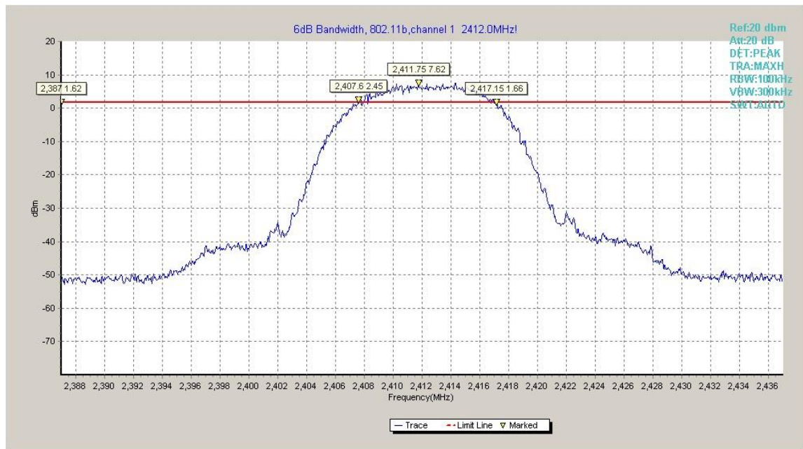
Fig.A.4.1 Occupied 6dB Bandwidth(802.11b,Ch 1)
