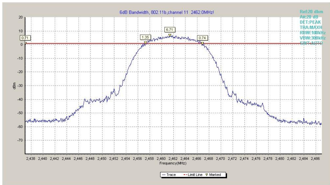
Fig.A.4.3 Occupied 6dB Bandwidth (802.11b, Ch 11)
