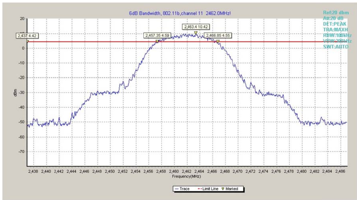
Fig.A.4.3 Occupied 6dB Bandwidth (802.11b, Ch 11)
