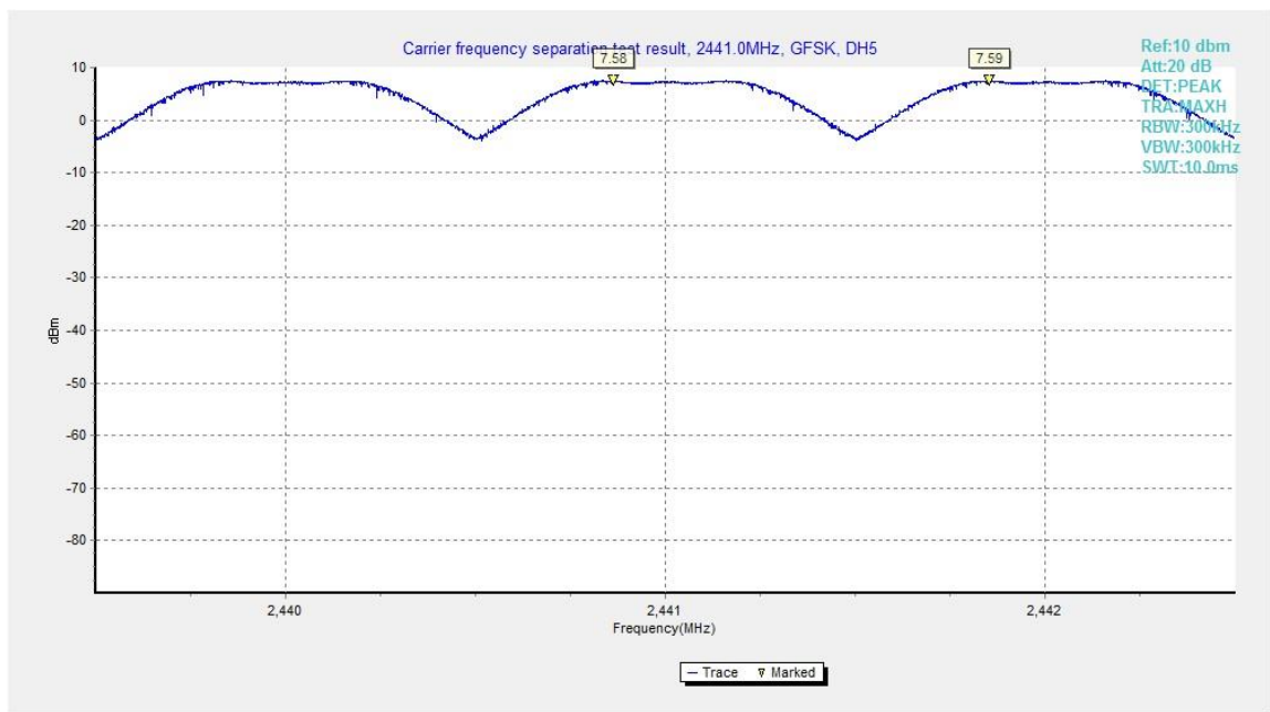
Fig.107. Carrier frequency separation measurement: GFSK, Channel 39
