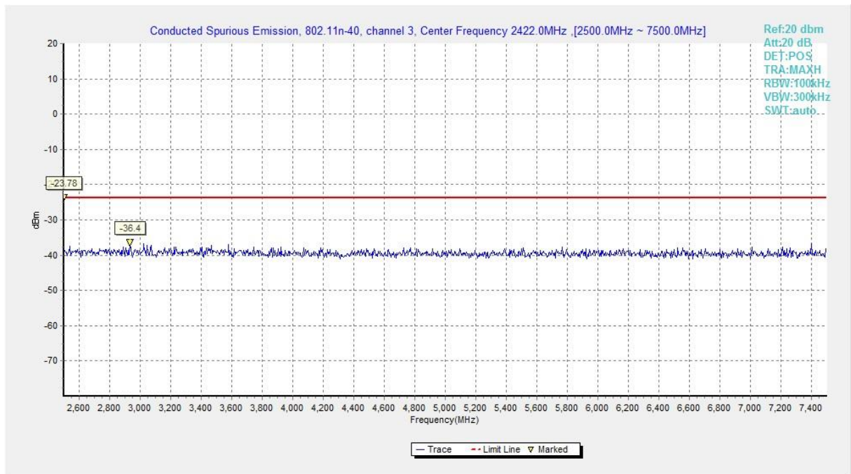
Fig.A.6.1.76 Transmitter Spurious Emission - Conducted (802.11n-HT40, Ch3, 2.5 GHz-7.5 GHz)
