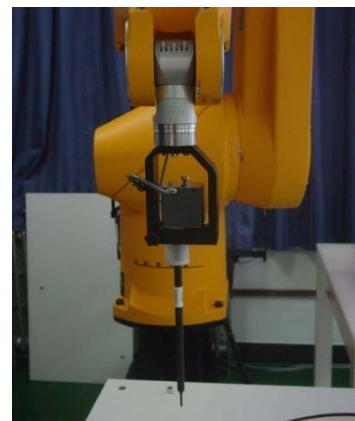
Picture C.3 E-field Probe
