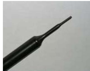
Picture C.2 Near-field Probe
