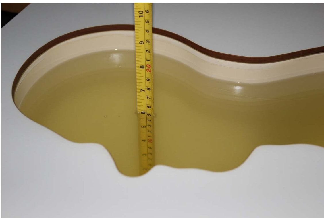
Picture 7-7 Liquid depth in the Head Phantom (1750 MHz)
